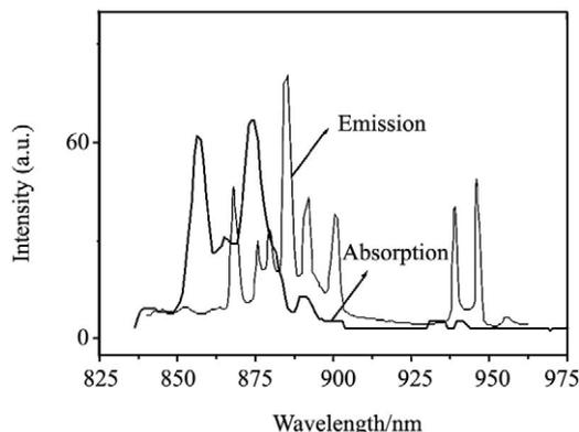
Fig.3 Absorption and emission spectra for  ${}^4I_{9/2} \leftrightarrow {}^4F_{3/2}$  transition of  $\text{Nd}^{3+}$  in YAG laser crystal at room temperature
