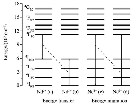
Fig.1 Cross-relaxation energy transfer and energy migration between Nd<sup>3+</sup> ions in YAG laser crystal
