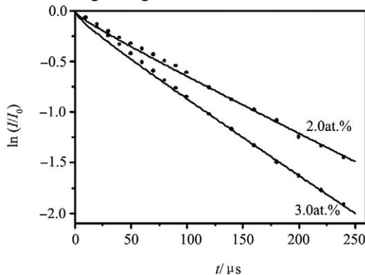
Fig.2 Luminescence decay curves of  ${}^4F_{3/2}$  level of  $\text{Nd}^{3+}$  in 2.0at.% and 3.0at.% doped YAG laser crystal at room temperature (The dots show the experimental results; the solid lines are the best fits obtained by application of the Y-T model for electronic dipole-electronic dipole interactions)
