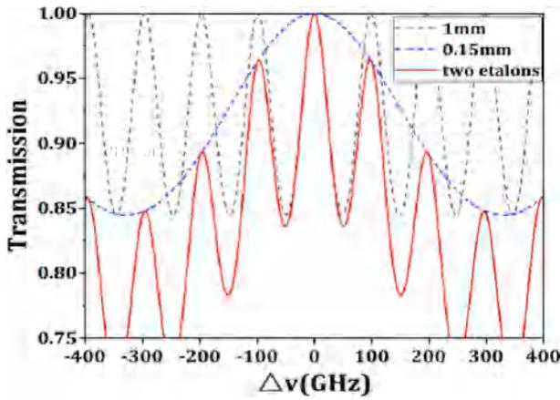
Fig. 3. The individual transmissions of F-P etalons with thicknesses of 1 mm and 0.15 mm (dashed curve) and combined transmission of two etalons (solid curve).
