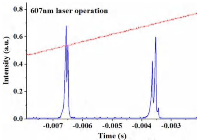
Fig. 4. A F-P interferometer scanning spectra of 607 nm laser with much reduced longitudinal mode numbers under the introduction of the 0.15-mm etalon.
