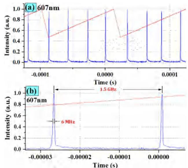
Fig. 6. (a) F-P interferometer scanning spectrum and (b) linewidth measurement of the 607 nm SLM laser.
