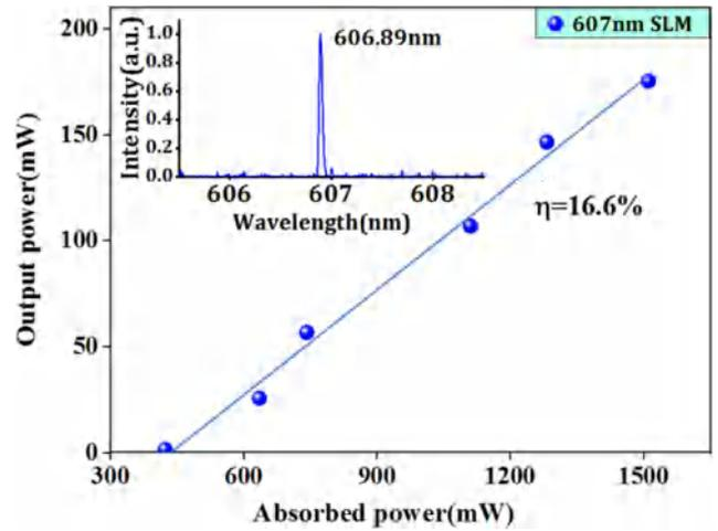
Fig. 5. Output power versus absorbed power of the SLM laser at 607 nm; Insets: the corresponding laser spectrum.
