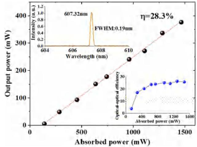
Fig. 2. Output power versus absorbed power for free-run 607 nm laser; inset: laser spectrum and the whole optical-optical efficiency.
