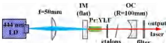
Fig. 1. Laser experimental setup of diode-pumped orthogonally polarized SLM Pr:YLF laser at 604 nm and 607 nm.
