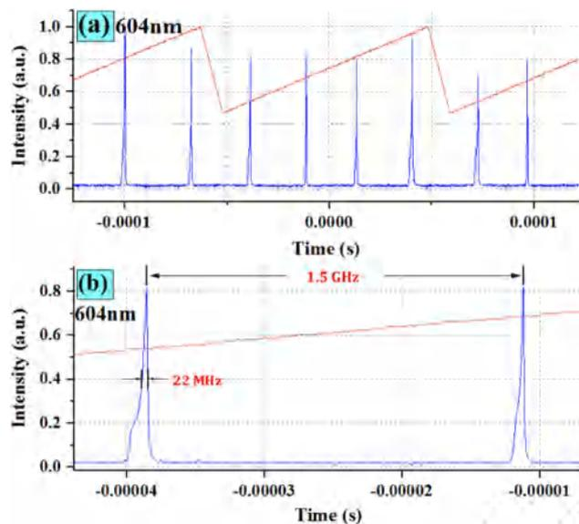
Fig. 8. (a) F-P interferometer scanning spectrum and (b) linewidth measurement of the 604 nm SLM laser.
