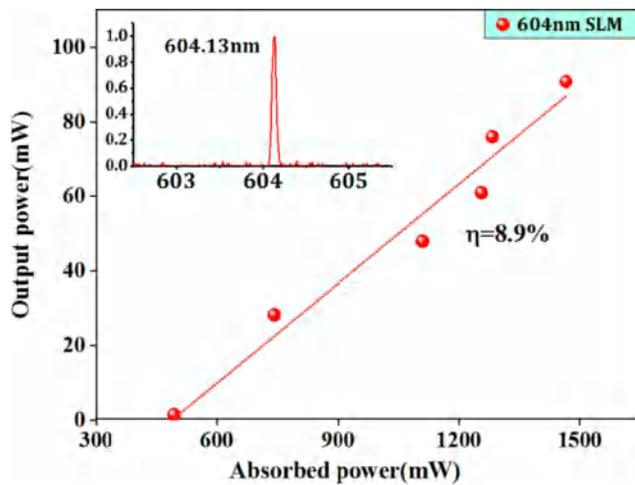
Fig. 7. Output power versus absorbed power of the SLM laser at 604 nm; Insets: the corresponding laser spectrum.
