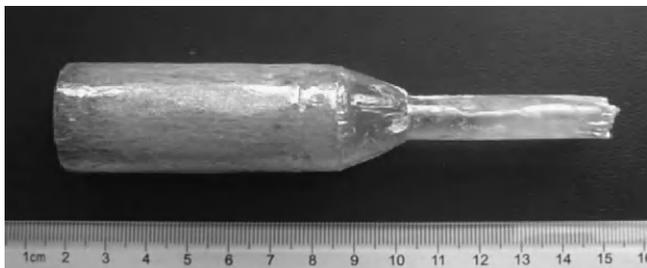
Fig. 4.  $\text{LaCl}_3:\text{Ce}^{3+}$  crystal grown by vertical Bridgman method.
