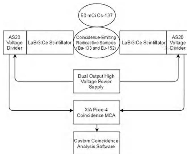
Fig. 1. LaBr<sub>3</sub>:Ce Block Diagram.
