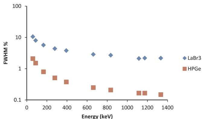
Fig. 5. A comparison of the energy resolution of LaBr<sub>3</sub>:Ce and HPGe detectors.
