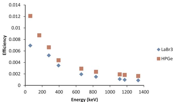
Fig. 4. A comparison of the efficiency of LaBr<sub>3</sub>:Ce and HPGe detectors.
