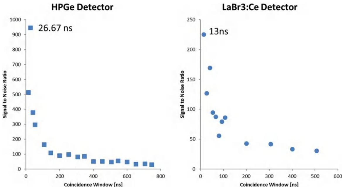
Fig. 3. SNR vs coincidence timing window for the HPGe and LaBr<sub>3</sub>:Ce detectors.
