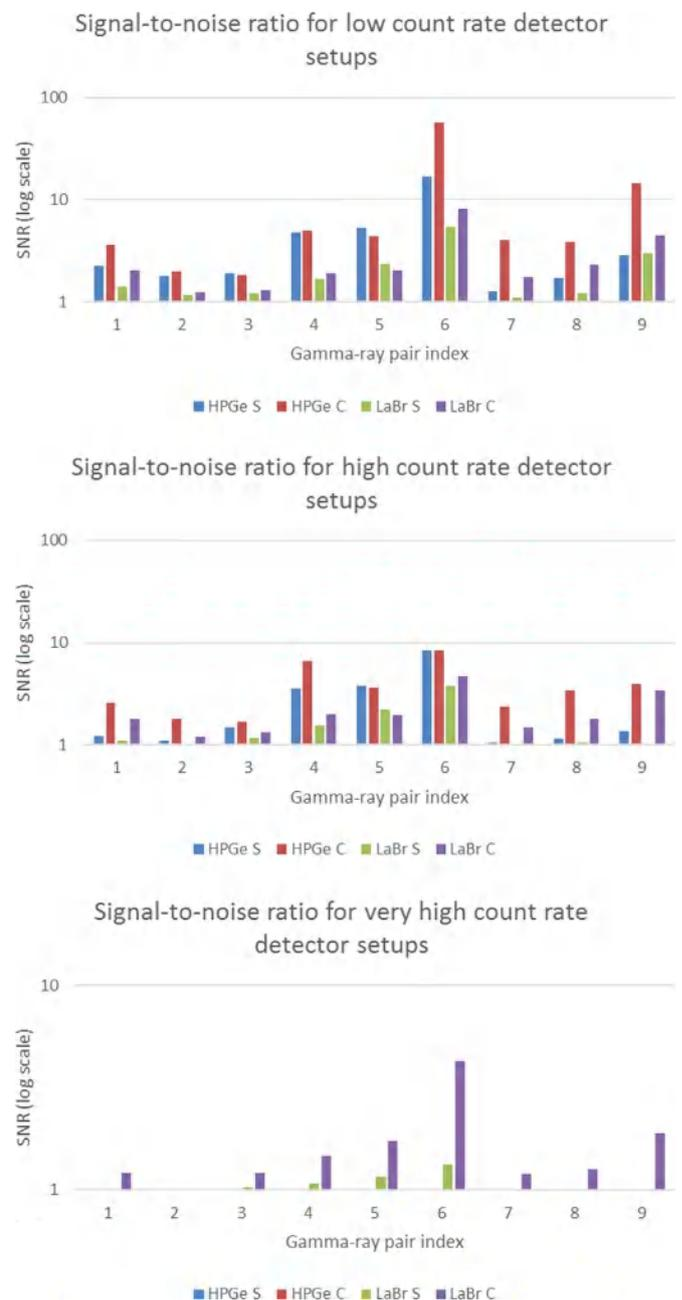
Fig. 7. Signal-to-noise ratios for all detector setups for low, high, and very high count rates. The pair of coincident gamma-rays corresponding to each index are the pairs of gamma-rays listed in Table 1 in order.
