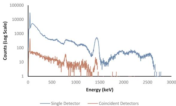
Fig. 6. Background spectrum characteristic of LaBr<sub>3</sub>:Ce detectors. The top curve represents a background spectrum collected with a single LaBr<sub>3</sub>:Ce detector. The bottom curve represents a background spectrum collected with coincident LaBr<sub>3</sub>:Ce detectors, with a coincidence gate applied over the energy range 5–2900 keV. (It should be noted that both curves represent the same dataset. The coincidence curve just applies additional gating logic.).
