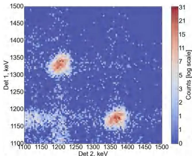
Fig. 2. <sup>60</sup>Co coincidence heatmap. The energy coordinates at (1173, 1173) and (1332, 1332) represent false coincidence events, while (1173, 1332) and (1332, 1172) represent true coincidence events.
