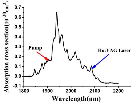
Fig. 2. Absorption cross section of Ho:SSO crystal.
