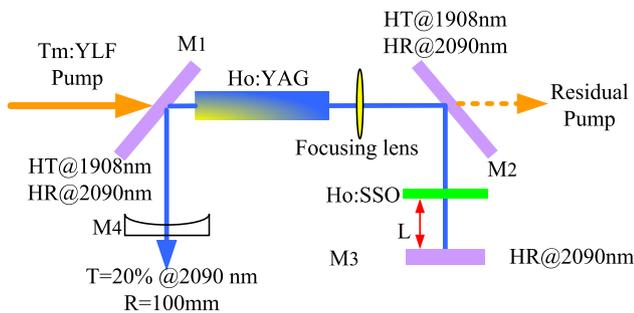
Fig. 1. Schematic diagram for the PQS Ho:SSO laser.
