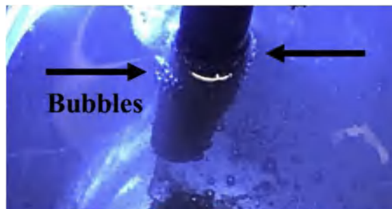
Fig. 5. Appearance around glassy carbon rod in the molten salt during applying the voltage.
