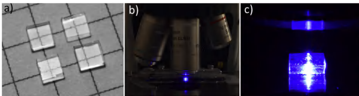
Fig. 1. LiF crystal samples: a) samples after polishing, b) a sample illuminated through the objective of the Nikon Eclipse Ni-U fluorescent microscope, c) a close-up of the illuminated sample.
