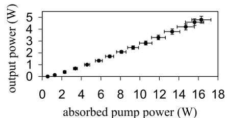
Fig. 2. Output power at 1322.6 nm versus absorbed pump power at 808 nm for standing-wave laser shown in Fig. 1 using an  $a$ -axis Nd:YLF crystal.
