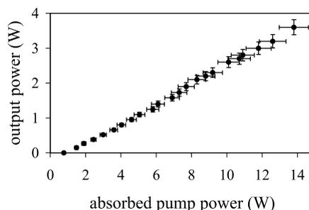
Fig. 4. Output power at 1312.0 nm versus absorbed pump power at 808 nm for a standing-wave laser shown in Fig. 1 with a  $c$ -axis Nd:YLF crystal.
