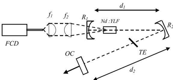
Fig. 1. Folded cavity standing-wave configuration for diode-pumped Nd:YLF laser used to generate 1312.0 and 1322.6 nm. Key: FCD, fibre-coupled diode; TE, Suprasil thin etalon; OC, output coupler ( $T = 2\%$ ). Here  $f_1 = 60$  mm,  $f_2 = 80$  mm,  $d_1 = 280$  mm,  $d_2 = 300$  mm,  $R_1 = 100$  mm, and  $R_2 = 500$  mm.
