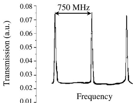
Fig. 3. Oscilloscope trace of transmission through a 0.75 GHz FSR confocal Fabry–Perot confirming single-frequency operation at 1322.6 nm of the standing-wave laser incorporating an intra-cavity etalon.
