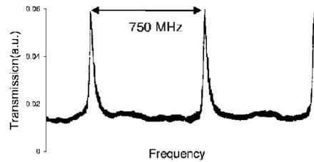
Fig. 6. Oscilloscope trace of transmission through a 0.75 GHz FSR confocal Fabry–Perot confirming single-frequency operation at 1312.0 nm of the twisted-mode folded-cavity laser incorporating an intra-cavity etalon (Fig. 5).
