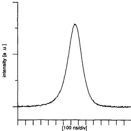
Fig. 7. Typical temporal profile of the Cr:LiSAF laser output pulse.
