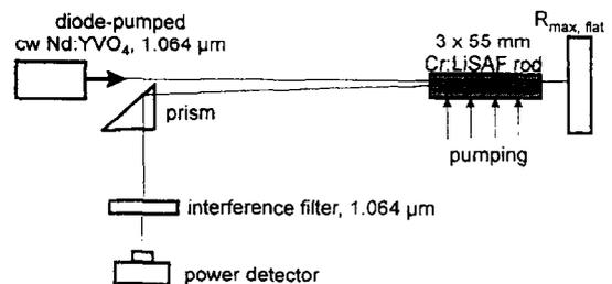
Fig. 9. Set-up for the determination of the transmission of the pumped and the unpumped Cr:LiSAF crystal.
