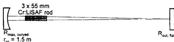
Fig. 1. Experimental set-up: Near-hemispherical resonator configuration, corresponding  $TEM_{00}$  mode and location of the Cr:LiSAF rod within the cavity.
