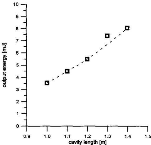
Fig. 5. Output energy versus cavity length for a reflectivity of the output coupler of  $R = 50\%$  for Nd:glass.
