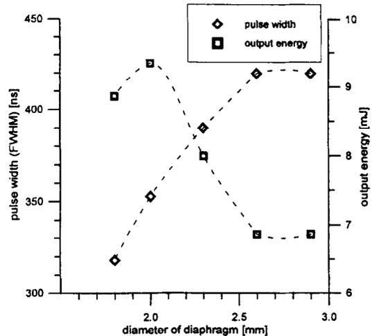
Fig. 11. Pulse width and corresponding output energy of the Cr:LiSAF laser versus the diameter of the inserted diaphragm.
