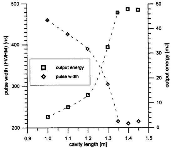
Fig. 4. Pulse width and corresponding output energy versus cavity length for a reflectivity of the output coupler of  $R = 50\%$  for Cr:LiSAF.
