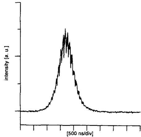
Fig. 8. Typical temporal profile of the Nd:glass laser output pulse.
