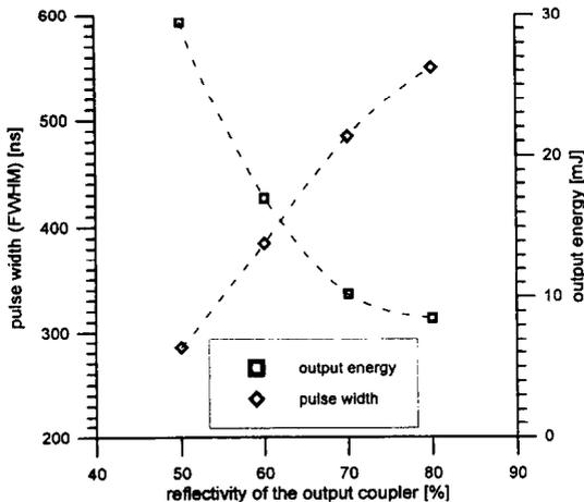
Fig. 3. Pulse width and corresponding output energy versus reflectivity of the output coupler for a cavity length of 1.25 m for Cr:LiSAF.
