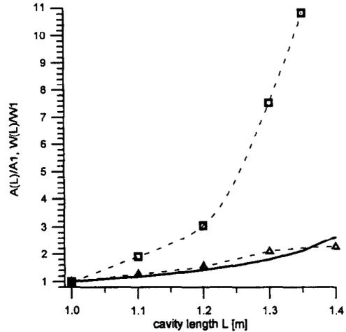
Fig. 6. Output energies  $W(L)$  normalized to  $W_1 = W(L = 1 \text{ m})$  for Cr:LiSAF (squares) and Nd:glass (triangles) and cross sections of the laser rod transmitted by the beam  $A(L)$  normalized to  $A_1 = A(L = 1 \text{ m})$  (solid line) versus cavity length.
