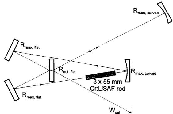
Fig. 2. Experimental set-up: Unidirectional ring resonator.
