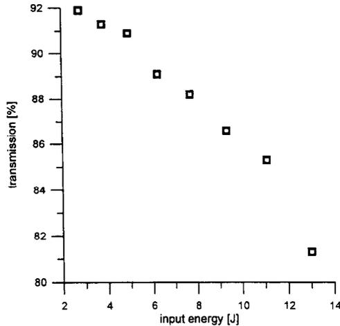
Fig. 10. Transmission of the pumped Cr:LiSAF versus the pump energy.
