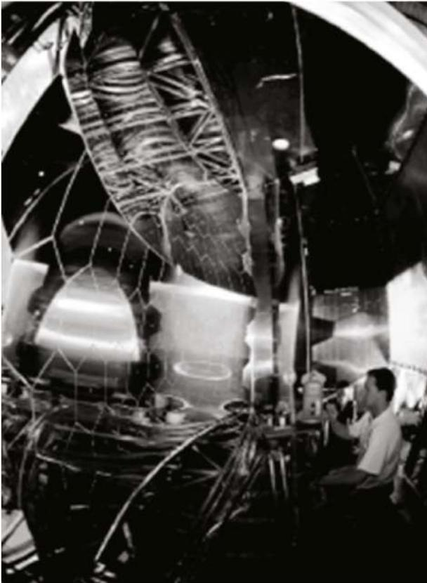
Fig. 5. The RICH mirror wall; the picture has been taken during the mirror alignment procedure [11].
