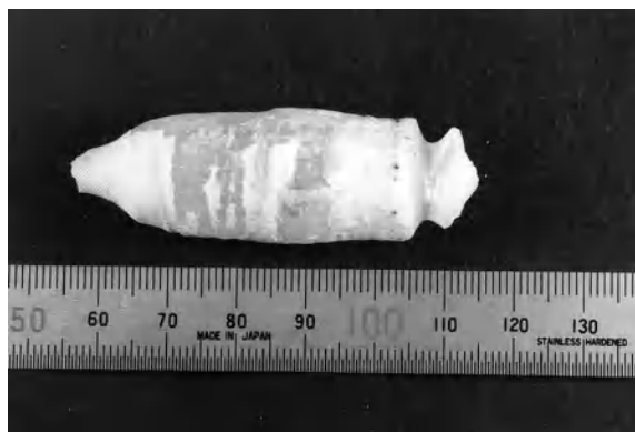
Fig. 1. As-grown Ce-doped \text{LiCaAlF}_6 single crystal pulled along the a -axis.
