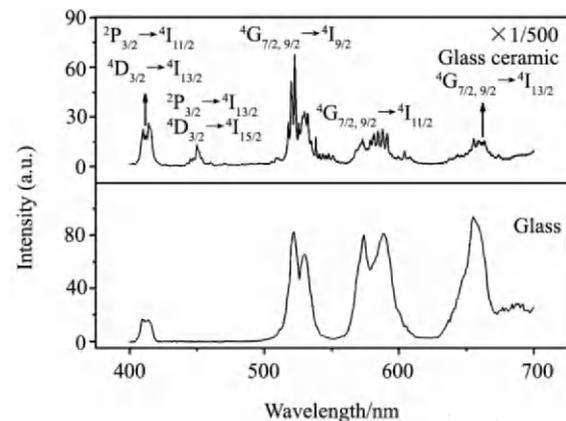
Fig.3 Room temperature upconversion emission spectra of the precursor glass and glass ceramic in the wavelength range of 400–700 nm
