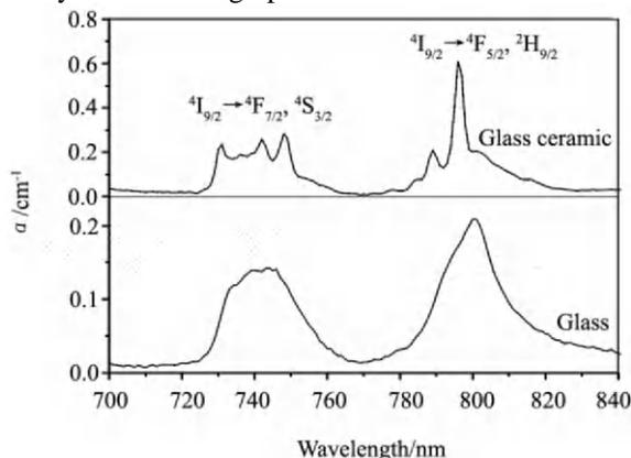
Fig.1 Room temperature absorption spectra of glass and glass ceramic
