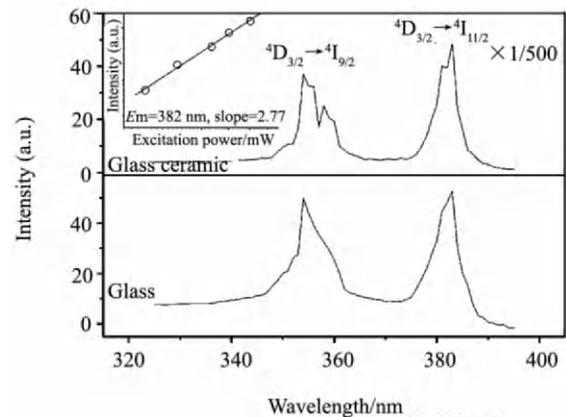
Fig.2 Room temperature upconversion emission spectra of the precursor glass and glass ceramic in the wavelength range of 320–400 nm, the inset shows the logarithmic plot of upconversion intensity versus excitation power
