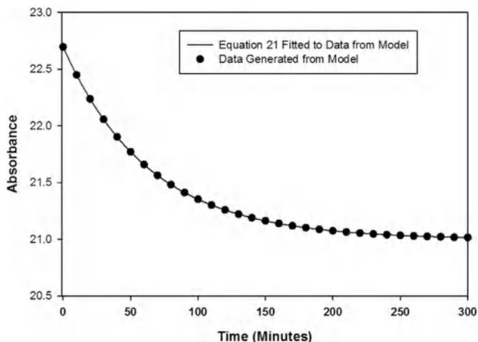
Fig. 3. Model of exponential decay of absorbed water in KBr disk containing solid biomaterial.
