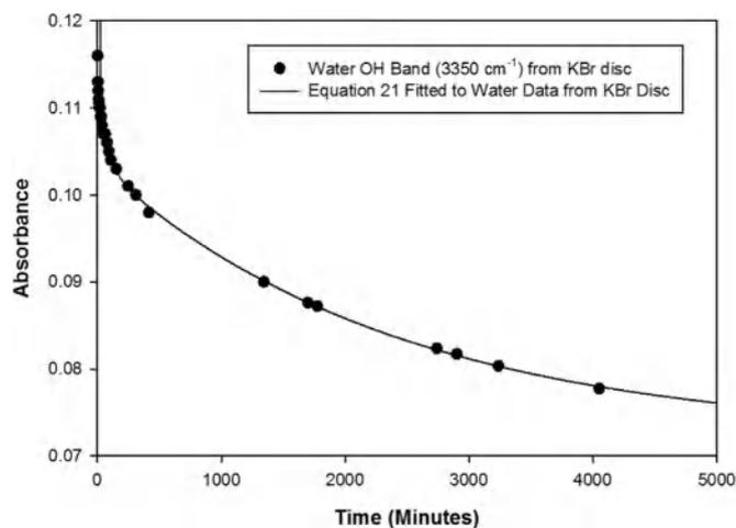
Fig. 5. Experimental exponential decay of water in blank KBr disk.
