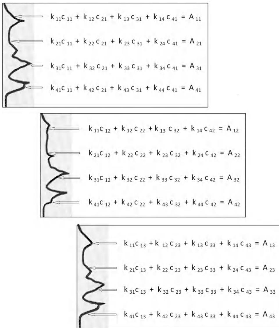
Fig. 1. FT-IR spectra of three mixtures of three components with Beer-Lambert law equations for absorbances at four frequencies.
