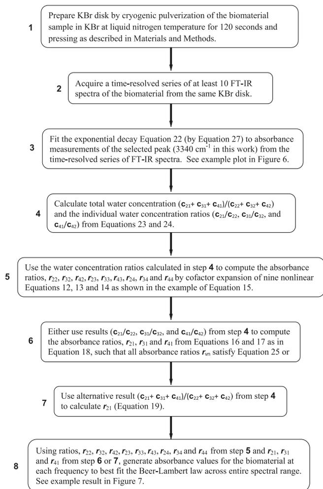
Fig. 4. Flowchart summarizing the eight main steps of the KBr water correction method.
