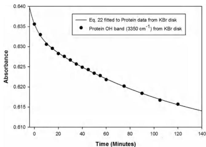
Fig. 6. Typical exponential decay of absorbed water in KBr disk containing solid protein.
