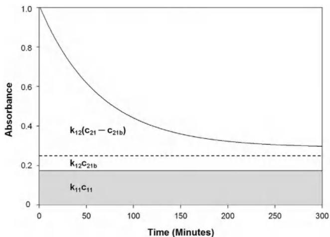
Fig. 2. Exponential decay of the absorbance of a theoretical solid biomaterial with one water band.
