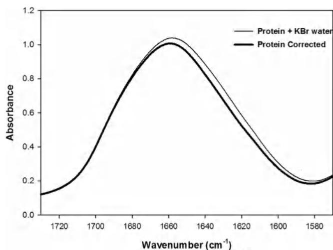
Fig. 7. FTIR spectra of protein in KBr before (gray) and after (black) water interference correction.
