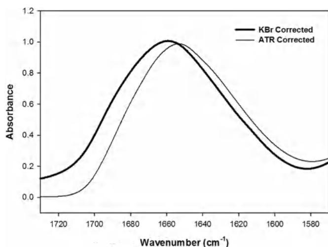
Fig. 8. Amide region of protein in KBr (black) after correction for water interference compared with amide region of protein by ATR (gray) after refractive index correction.
