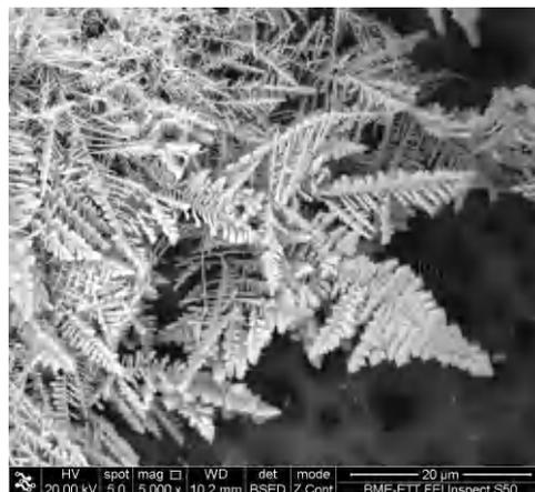
Fig. 1. Scanning electron microscope (SEM) image of dendrites.
