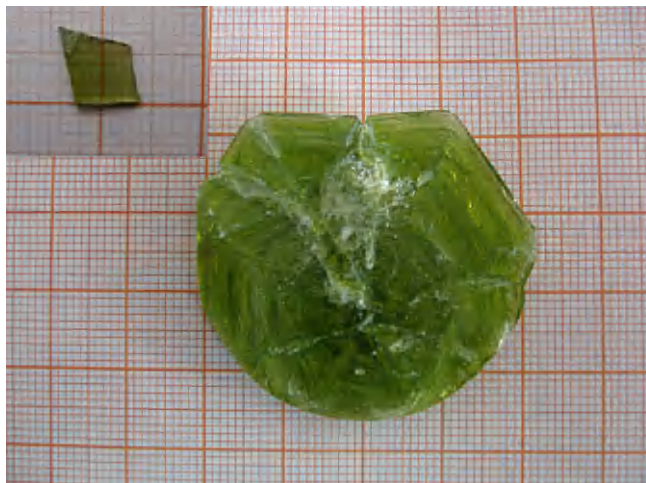
Fig. 2. Photograph of the grown Cr 3+ :CsAl(MoO 4 ) 2 crystal.
