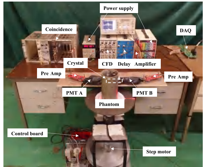
Fig. 7. Experimental setup of the computed tomography.
