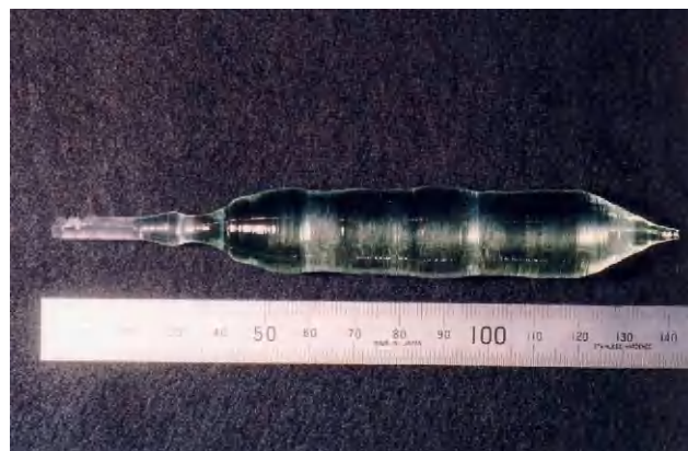
Fig. 1. 10% \text{Yb}^{3+} -doped \text{YLiF}_4 single crystal with 1 in. in diameter grown by the Czochralski method.
