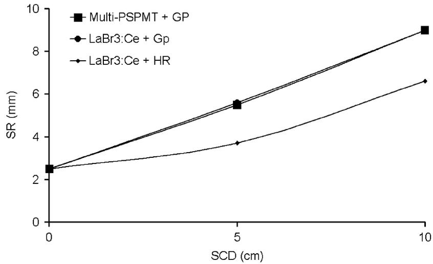
Fig. 2. Spatial resolution vs. source-to-collimator distance for both the cameras.
