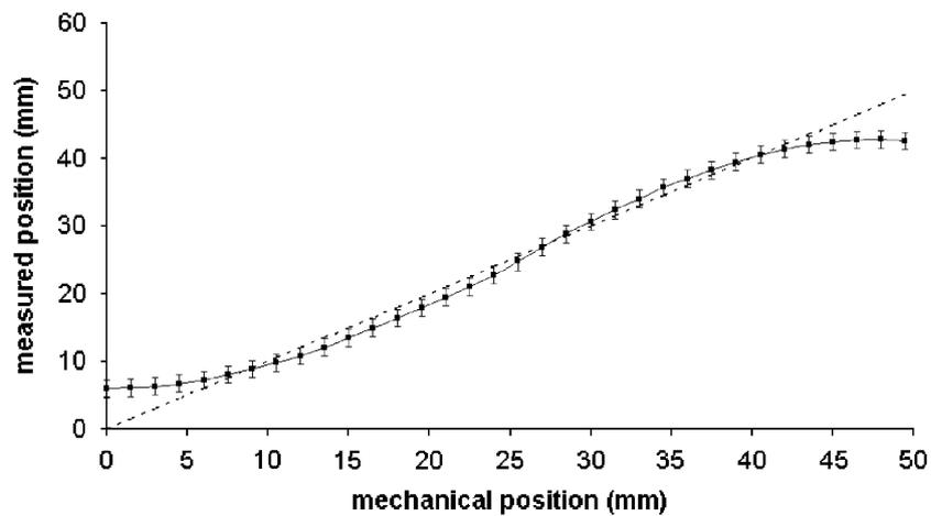
Fig. 3. Linearity Range of LaBr3:Ce  $\gamma$ -camera.
