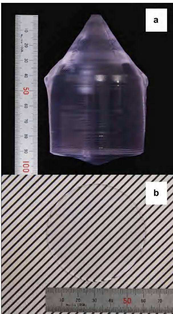
Fig. 2. View of as-grown Nd:LiLuF 4 single crystal (a) and disk cut from the crystal (b).
