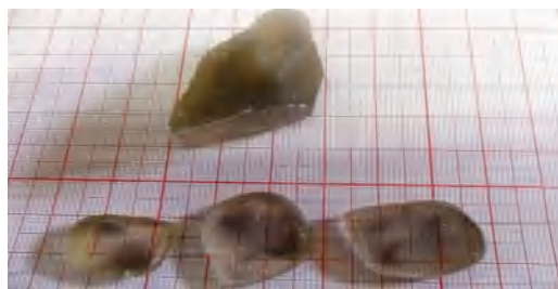
Fig. 1. Photograph of a KBr:CuO single crystal.
