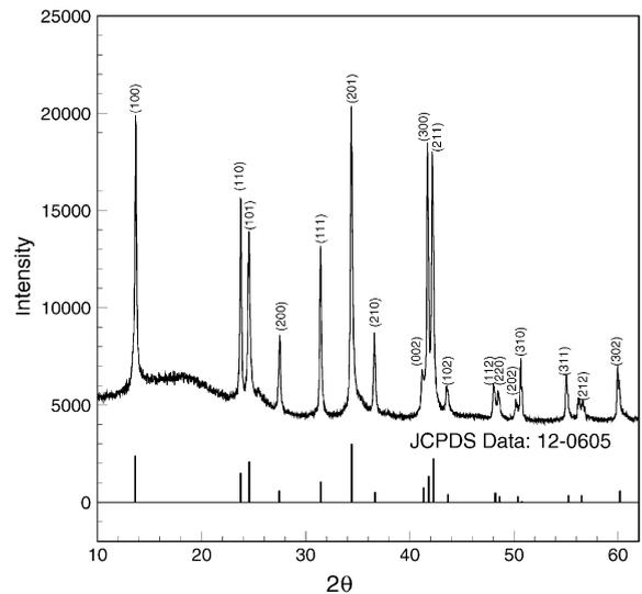
Fig. 2. XRD pattern of as-grown  $\text{LaCl}_3$  crystal.
