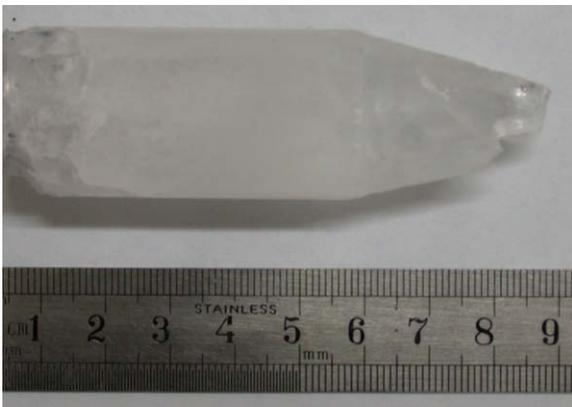
Fig. 1. As-grown  $\text{LaCl}_3$  crystal by Modified Bridgman Method.
