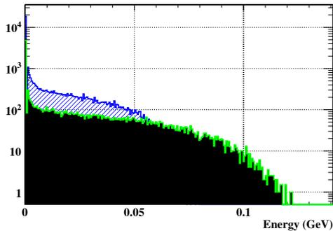
Figure 5: Monte Carlo simulation. Energy loss in the  $3'' \times 3''$   $\text{LaBr}_3(\text{Ce})$  for  $\gamma$  in the  $55 \div 83$  MeV energy interval (blue) and at an energy of 129 MeV (green).
