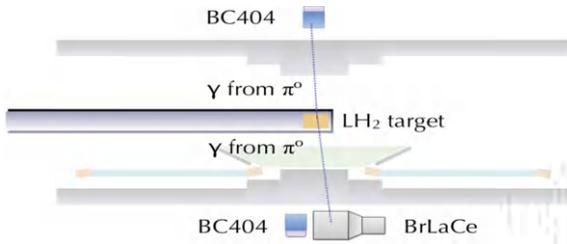
Figure 1: Test setup (side view). The  $\pi^-$  are stopped into the LH<sub>2</sub> target and back-to-back events can be detected by the Top BC404 detector and the Bottom LaBr<sub>3</sub>(Ce) detector.
