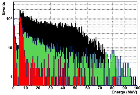
Figure 4: The collected charge on the  $\text{LaBr}_3(\text{Ce})$  detector for the three categories of events:  $\gamma$  in the  $55 \div 83$  MeV energy interval (blue),  $\gamma$  at an energy of 129 MeV (green) and neutrons at 9 MeV (red).
