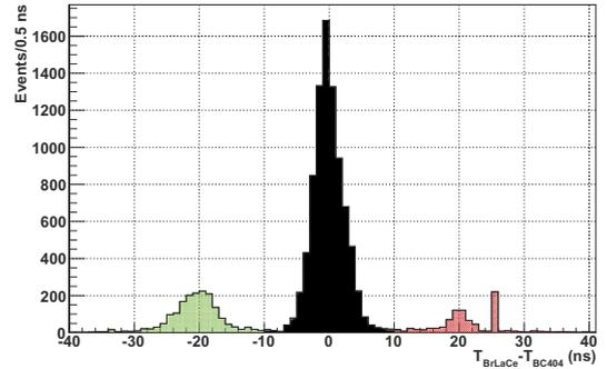
Figure 2: Time structure for back-to-back events selected with the LaBr<sub>3</sub>(Ce) crystal and the Top BC404.
