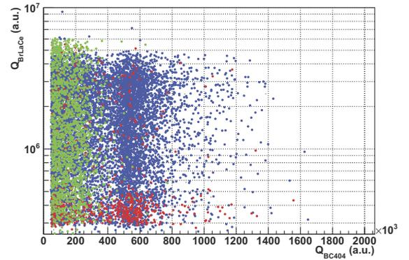
Figure 3: The collected charge on the LaBr<sub>3</sub>(Ce) detector versus the BC404 detector selecting the three categories of events by means of timing cut:  $\gamma$  in the 55 ÷ 83 MeV energy interval ( $|\Delta T| < 10$  ns, blue),  $\gamma$  at an energy of 129 MeV and neutrons at 9 MeV, with  $n$  into the LaBr<sub>3</sub>(Ce) ( $\Delta T > 10$  ns, red) and  $n$  into the BC404 ( $\Delta T < -10$  ns, green).
