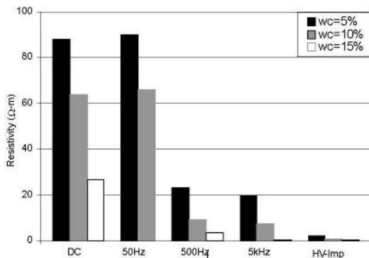
Figure 12: Wet NaCl resistivity values for different applied voltage types.
