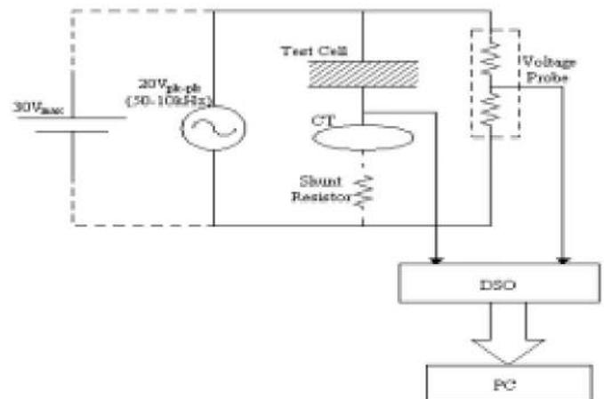
Figure 1: Test circuit for AC and DC characterisations.
