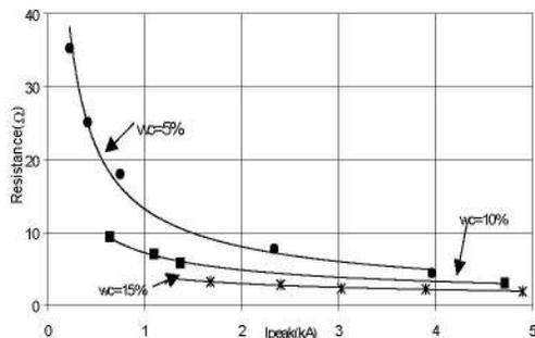
Figure 11: Resistances ( $\Omega$ ) vs current peak (kA) for wet NaCl.
