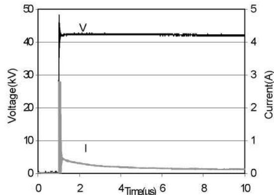
Figure 9: Voltage and current traces of dry NaCl at charging voltage of 43kV.
