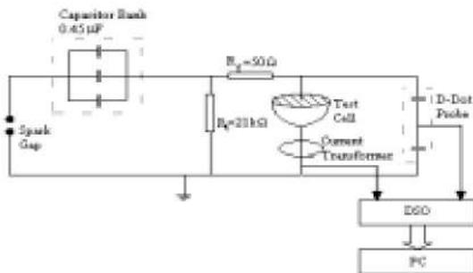
Figure 8: Impulse test circuit
