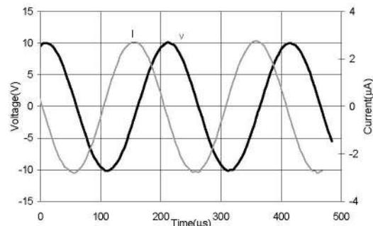
Figure 3: Voltage and current wavelshapes for AC tests on air gap at 1kHz.
