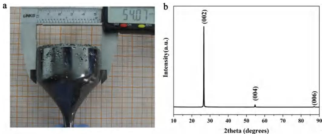
Fig. 1. (a) Photograph and (b) XRD pattern of CdSe single crystal.
