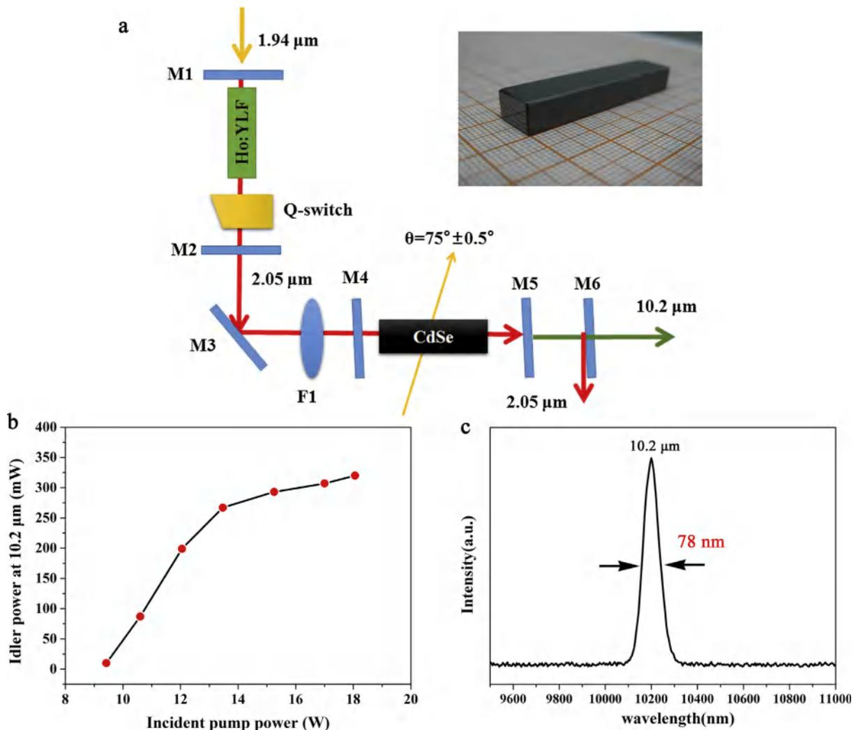
Fig. 3. (a) Schematic diagram of the OPO system, (b) Output powers of the idler, (c) Spectrum of the idler with the peak at 10.20  $\mu\text{m}$ .
