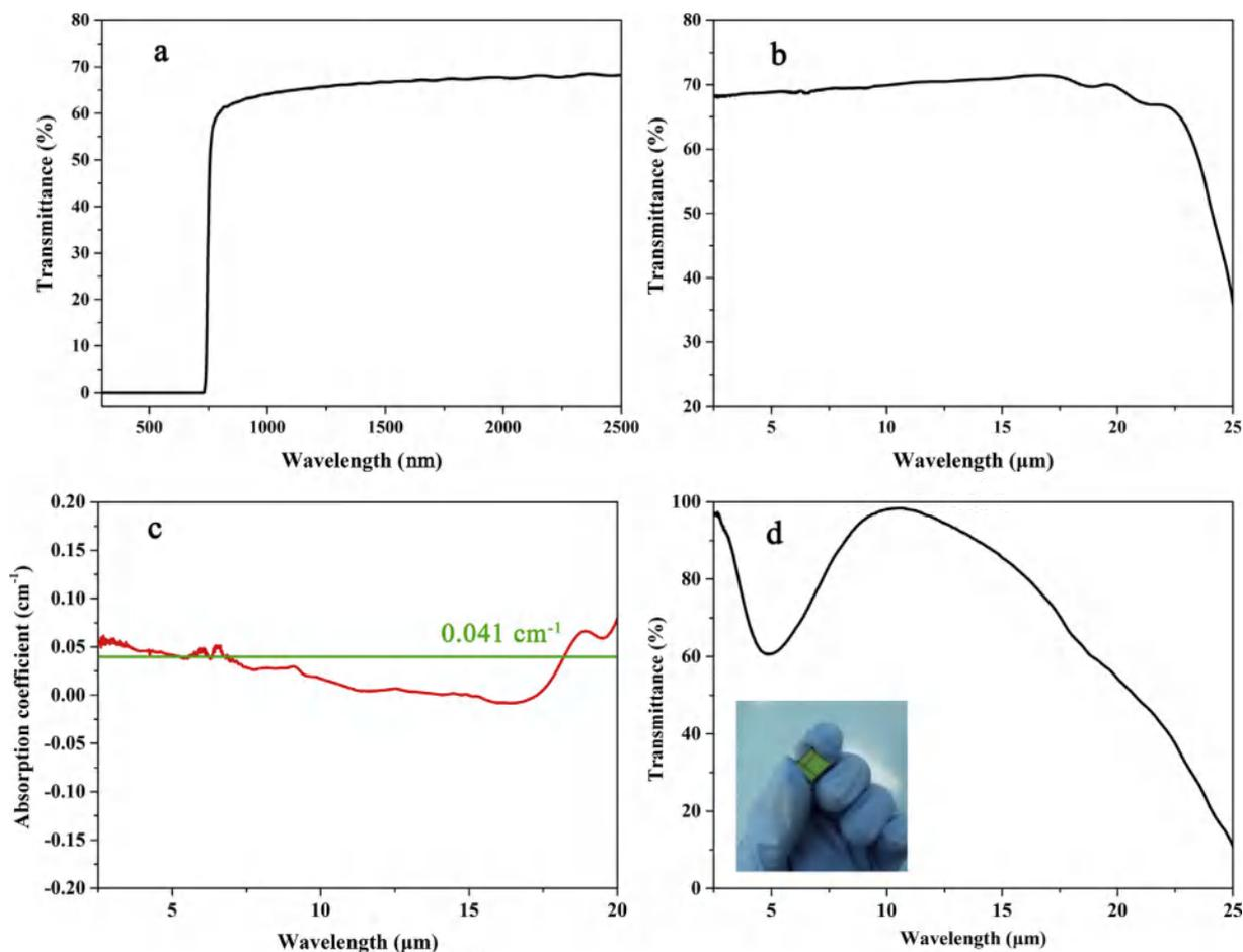
Fig. 2. (a) UV-Vis-NIR spectrum, (b) transmission spectrum without coating, (c) absorption coefficient without coating, (d) transmission spectrum with coating of the 4 mm thick CdSe crystal. The inset is photograph of 4 mm thick CdSe crystal with coating.
