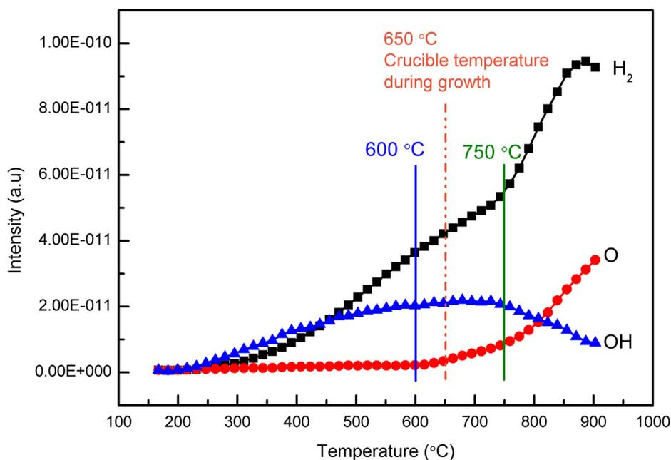
Fig. 4b. RGA analysis of residual gases and evolution of H<sub>2</sub> (-■-), O (-●-) and OH (-▲-) as a function of temperature during annealing of silica crucible.
