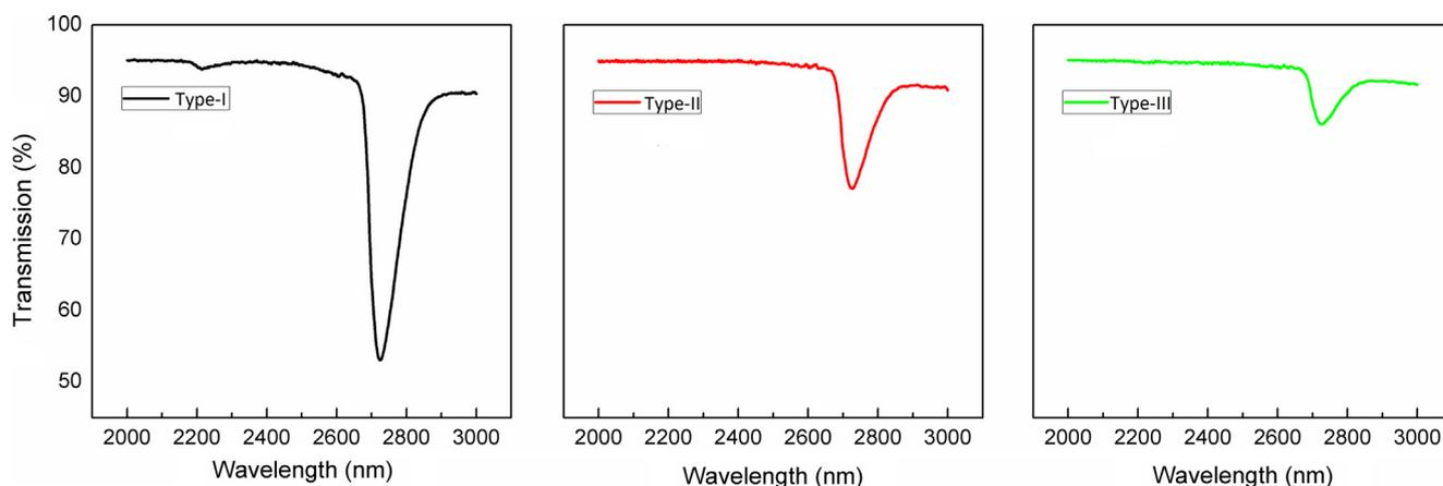
Fig. 2b. NIR Transmission spectra of silica glass crucibles used for the growth of Type-I, Type-II and Type-III crystals (Absorption peak at  $\sim 2730$  nm corresponds to OH and its intensity is proportional to amount of OH in quartz).
