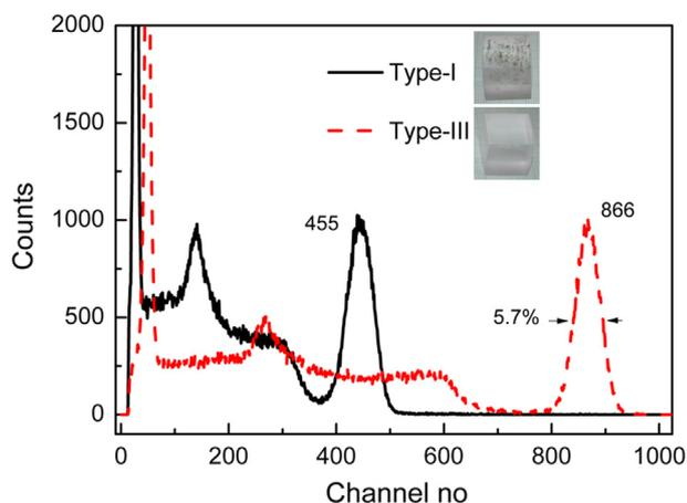
Fig. 5a. Pulse height spectra of  $^{137}\text{Cs}$  recorded using Type-I and III crystals as detector (sample size:  $20 \times 20 \times 20 \text{ mm}^3$ , shaping time:  $10 \mu\text{s}$ ).
