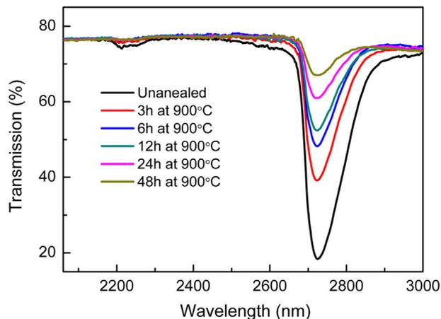
Fig. 4c. Absorption spectra of Silica glass for different annealing time at 900 °C showing the change in OH with annealing.
