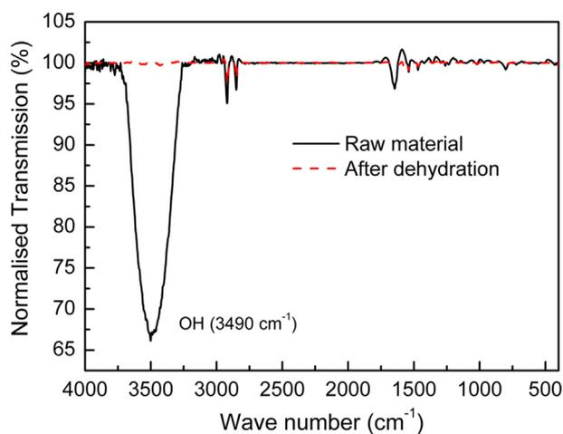
Fig. 3a. IR transmission spectra ( $450\text{--}4000\text{ cm}^{-1}$ ) of raw material, before (solid black line) and after dehydration (dashed red line). 3 mm thick pellets prepared by cold compaction were used for the measurements.
