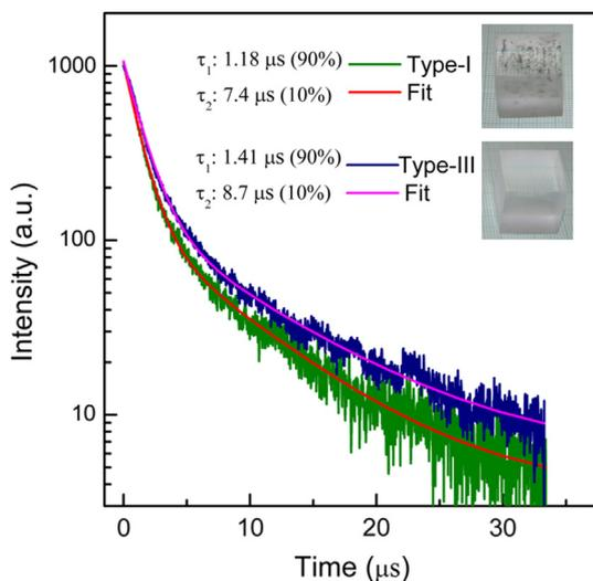
Fig. 5b. Decay profile of Type-I and III crystals (sample size:  $20 \times 20 \times 20 \text{ mm}^3$ , gamma source:  $^{137}\text{Cs}$ ).
