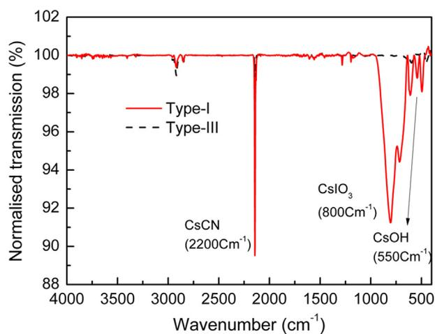
Fig. 3b. IR transmission spectra ( $450\text{--}4000\text{ cm}^{-1}$ ) of 3 mm thick discs of Type-I (solid red line) and Type-III (dashed black line) crystals.
