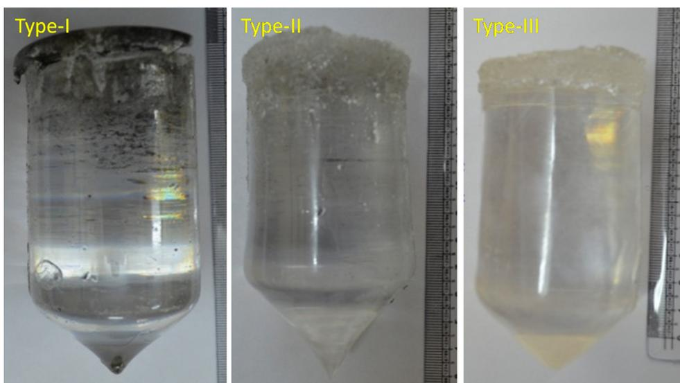
Fig. 2a. Photograph of CsI single crystals grown in quartz crucible containing OH in decreasing order form Type-I to Type-III.
