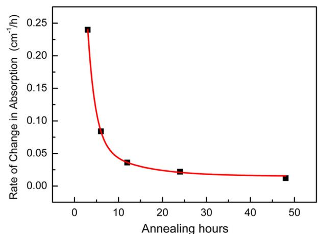
Fig. 4d. Rate of change in OH related absorption as a function of annealing time.
