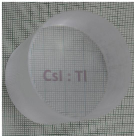
Fig. 6a. Scintillator detector (dia: 45 mm, L: 48 mm) fabricated using crystal grown under optimum condition (OH content in crucible  $< 10 \text{ ppm}$ ).
