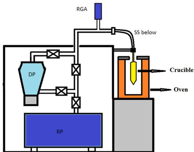
Fig. 4a. Schematic of the arrangement of RGA for measurements of residual gas composition during baking of silica glass crucible.
