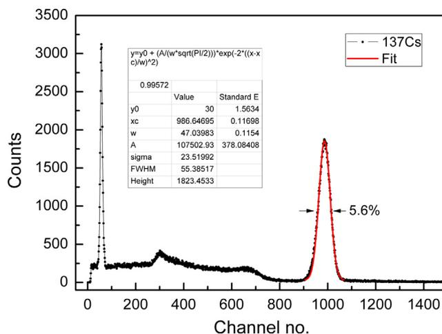
Fig. 6b. A gamma spectrum of  $^{137}\text{Cs}$  showing 5.6% resolution at 662 keV recorded by fabricated detector (dia: 45 mm, L: 48 mm).
