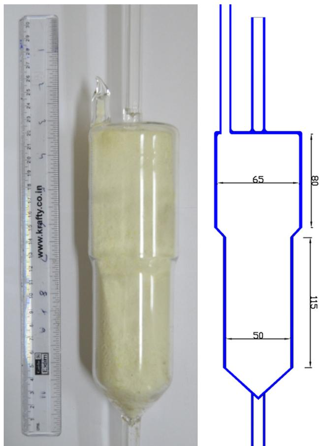
Fig. 1. Photograph of quartz crucible loaded with dehydrated material and sealed under vacuum ( $1 \times 10^{-5}$  mbar) along with the schematic drawing.
