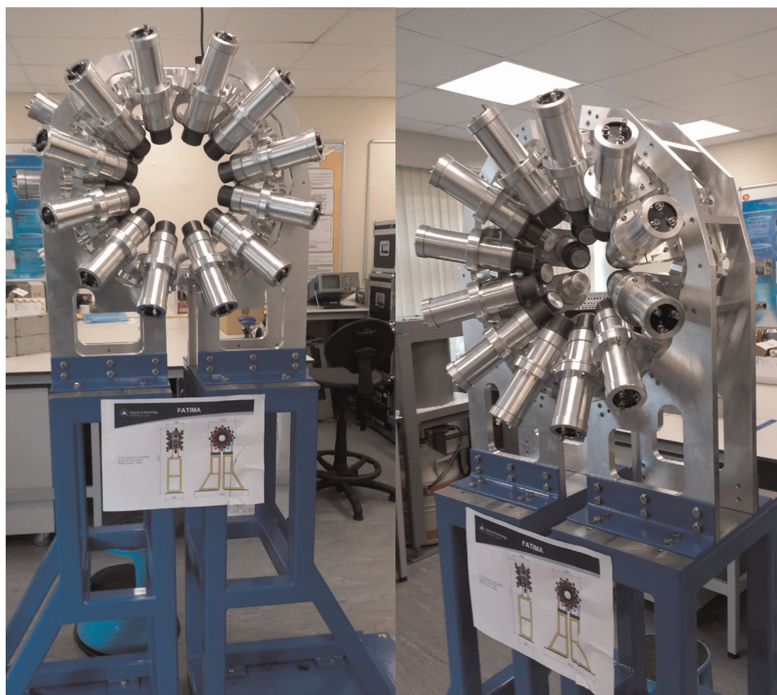
Fig. 1. Photographs of the support frame for the decay spectroscopy FAST-TIMing Array (FATIMA) of LaBr 3 detectors for future use within the DESPEC project at FAIR (Regan, 2012).
