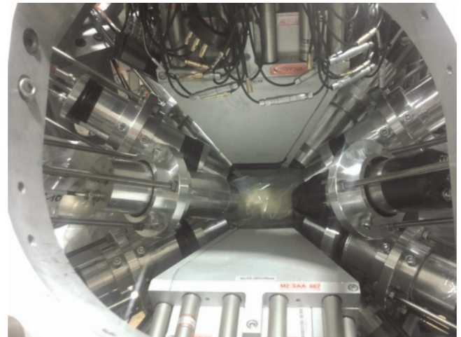
Fig. 5. Photograph of the target position of the EXILL + FATIMA set-up at ILL-Grenoble. This array combined the clover HpGe detectors in the EXOGAM array with 16 LaBr 3 detectors for fast-timing measurements of prompt fission fragments.
