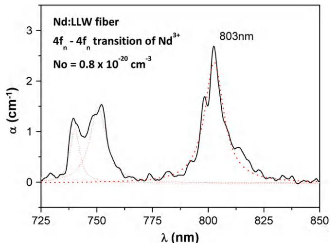
Fig. 2. Non-polarized absorption spectra of Nd:LLW single crystal fiber.
