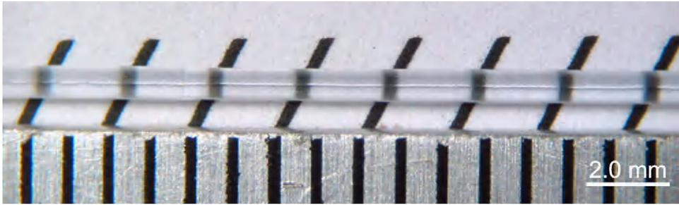
Fig. 3. As-grown single crystal fiber of YLF doped with 1.5 mol% Nd<sup>3+</sup>.
