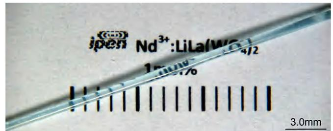
Fig. 1. As-grown Nd<sup>3+</sup>:LLW single-crystalline fiber doped with 1 mol%.
