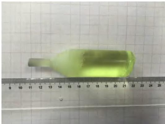
Fig. 1. Picture of the 0.6at.%Pr: $\text{Ca}_{0.94}\text{Gd}_{0.06}\text{F}_{2.06}$  crystal sample as grown.
