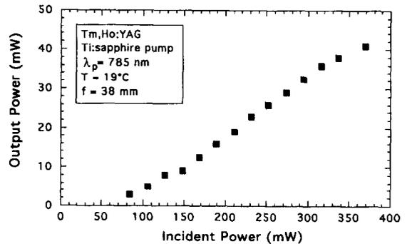
Fig. 3. Output power versus incident power for the  $\text{Tm,Ho:YAG}$  CW laser in the case of  $\text{Ti:Al}_2\text{O}_3$  laser pumping.
