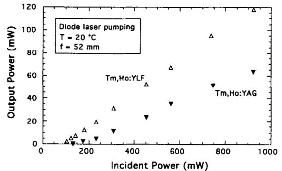
Fig. 4. Output power versus incident power for the Tm,Ho:YLF and the Tm,Ho:YAG CW lasers in the case of diode laser pumping. Pumping wavelengths are 792 and 785 nm for the YLF and YAG crystals, respectively.
