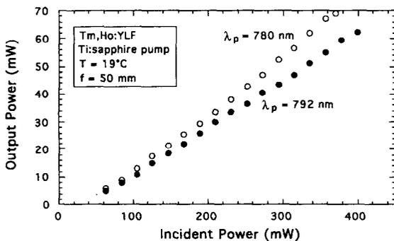
Fig. 2. Output power versus incident power for the  $\text{Tm,Ho:YLF}$  CW laser in the case of  $\text{Ti:Al}_2\text{O}_3$  laser pumping at two different wavelengths.
