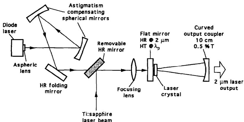
Fig. 1. Schematic of the resonator and pumping geometry used for the  $2\ \mu\text{m}$  laser characterization.
