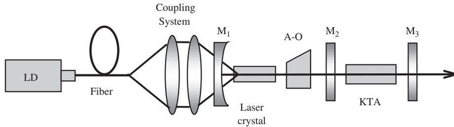
Fig. 2. Experimental setup of KTA IOPO.
