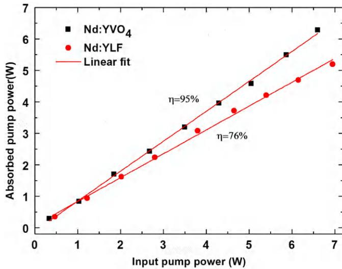
Fig. 3. Absorbed pump power for Nd:YVO<sub>4</sub> (a) and Nd:YLF (b).
