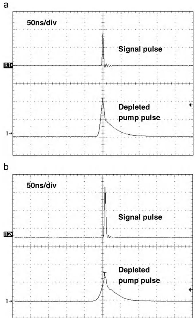
Fig. 8. Temporal behavior of the signal and depleted pump pulses pumped by Nd:YVO<sub>4</sub> (a) and Nd:YLF (b) lasers.
