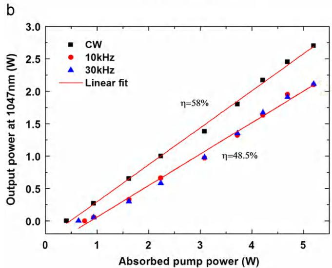
Fig. 4. Performance of Nd:YVO<sub>4</sub> (a) and Nd:YLF (b) lasers.
