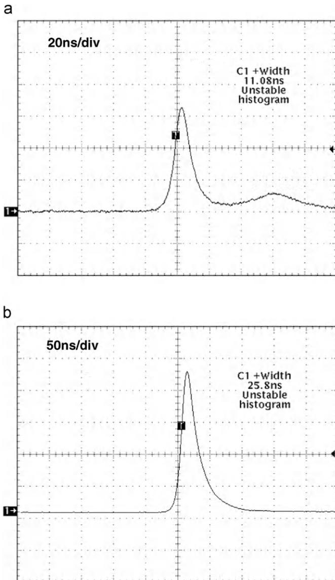
Fig. 5. Temporal behavior of Nd:YVO<sub>4</sub> (a) and Nd:YLF (b) laser pulses.
