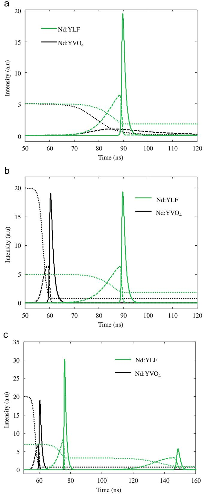
**Fig. 1.** Temporal characteristics of the KTA IOPO pumped by Nd:YVO<sub>4</sub> and Nd:YLF lasers. Inversion population—dotted curve; pump pulse—dashed curve; signal pulse—solid curve.
