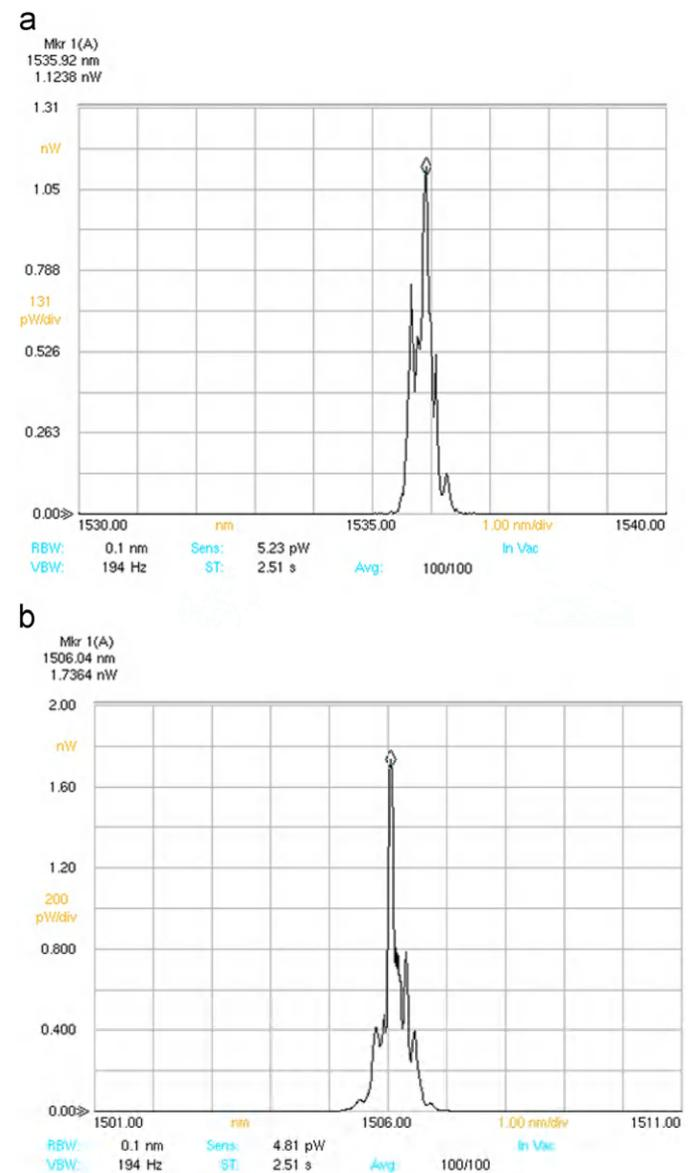
Fig. 6. Output spectrum of KTA OPO pumped by Nd:YVO<sub>4</sub> (a) and Nd:YLF (b) lasers.
