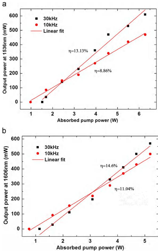
Fig. 7. Output signal power of KTA OPO pumped by Nd:YVO<sub>4</sub> (a) and Nd:YLF (b) lasers.
