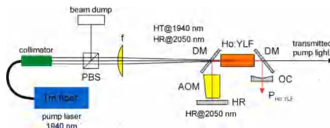
**Fig. 1.** Experimental setup of the end-pumped Ho:YLF laser: PBS – polarizing beam splitter, DM – flat dichroic mirrors anti-reflective at  $1.94\ \mu\text{m}$  and 45-deg highly reflective at  $2.05\ \mu\text{m}$ , OC – concave output-coupling mirror, AOM – acousto-optic modulator, HR – high reflector.
