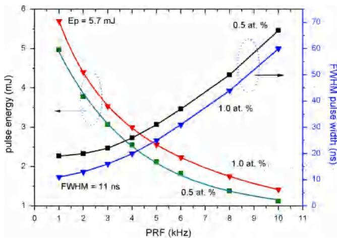
Fig. 3. Pulse energy and pulse width as a function of pulse repetition rate for the maximum pump power of 32.5 W.
