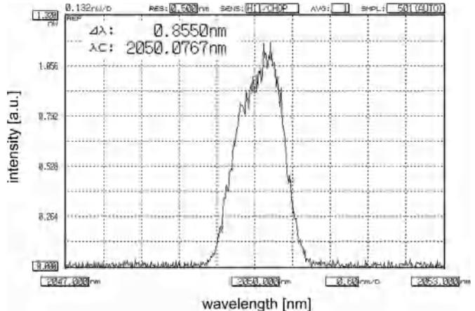
Fig. 5. Emission spectra of the Q-switched 1.0 at.% Ho:YLF laser.
