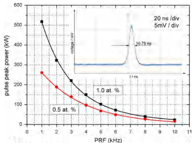
Fig. 4. Pulse peak power as a function of the pulse repetition rate for the maximum pump power of 32.5 W. The inset shows the scope of the shortest (10.75 ns) recorded pulse.
