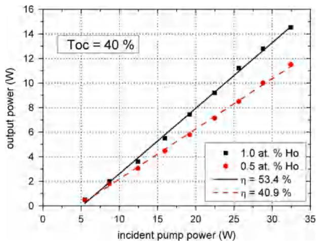
Fig. 2. Output powers of Ho:YLF lasers as a function of incident pump power for a lasers operating in the CW regime. The results of a linear fit and the calculated slope efficiencies are given in the graph.
