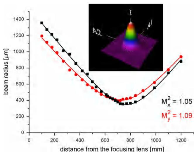
**Fig. 6.** Caustic determination for the Ho:YLF laser at the 5 kHz PRF and maximum pump power. The inset shows a spatial distribution of the Q-switched Ho:YLF laser beam.
