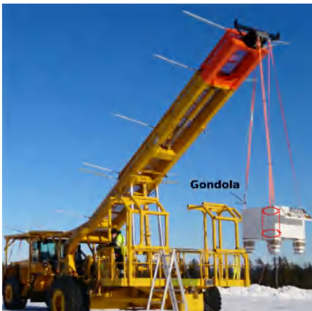
Fig. 7. The PoGOLino gondola before launch hanging from the launch vehicle. The position of PoGOLino is indicated with the dotted red lines. (For interpretation of the references to color in this figure caption, the reader is referred to the web version of this article.)
