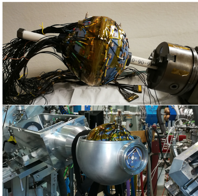
Fig. 4. Cabled CsI ball array, before (top) and after (bottom) insertion into the TIP chamber.
