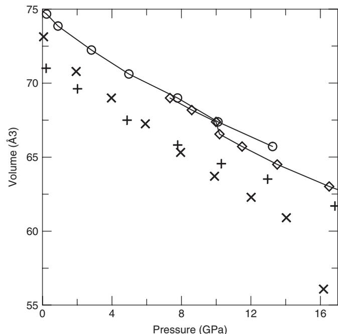
Fig. 5. Volume (per formula unit) versus pressure for the I<sub>41/a</sub> scheelite (circles) and P<sub>21/c</sub> M'-fergusonite (diamonds) structures. Experimental results after Ref. [5] (plus signs) and theoretical results after Ref. [6] (crosses) are also shown for comparison.
