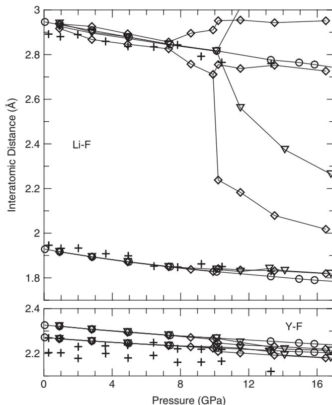
Fig. 7. Evolution with the pressure of the interatomic distances below 3 Å between Li and F (upper panel), and Y and F (lower panel) neighbours in the scheelite structure (circles), the M-fergusonite (triangles), and the M'-fergusonite (diamonds). Experimental results after Ref. [5] (plus signs) are also shown for comparison.
