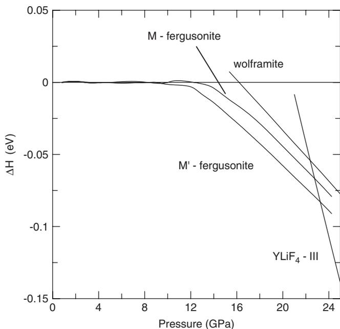
Fig. 4. Variation of enthalpy (per formula unit) with pressure. The enthalpy of the scheelite phase has been taken as reference. The post fergusonite stable structure proposed by Sen et al. is marked as YLiF<sub>4</sub>-III.
