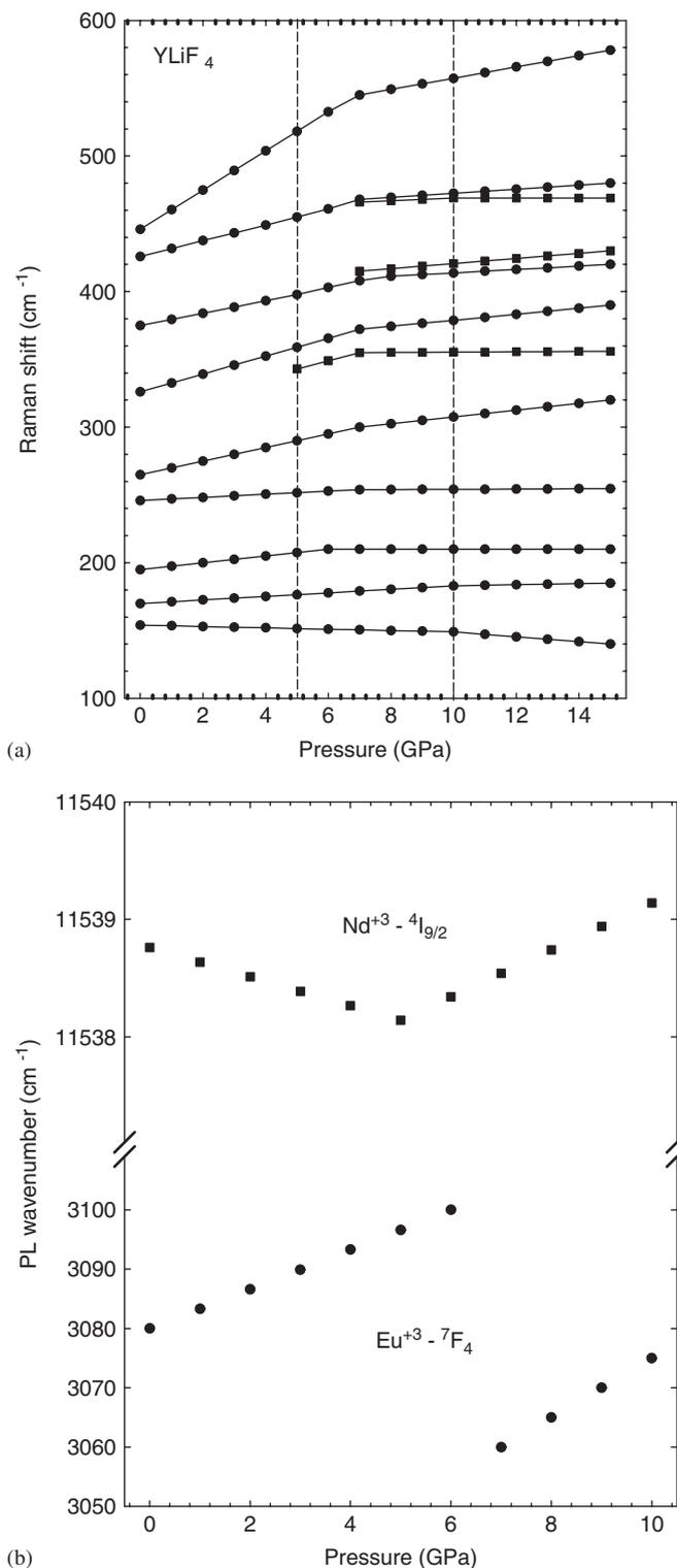
Fig. 6. (a) Pressure dependence of the Raman shifts in YLiF<sub>4</sub> at 300 K, after Refs. [2,4]; (b) Pressure dependence of the PL wavenumber of the <sup>7</sup>F<sub>4</sub> level of Eu<sup>3+</sup> at 300 K (after Ref. [1]), and of the <sup>4</sup>I<sub>9/2</sub> level of Nd<sup>3+</sup> at 5 K (after Ref. [3]). Changes of the Raman and photoluminescence frequencies between 5 and 7 GPa are evident in the figures.
