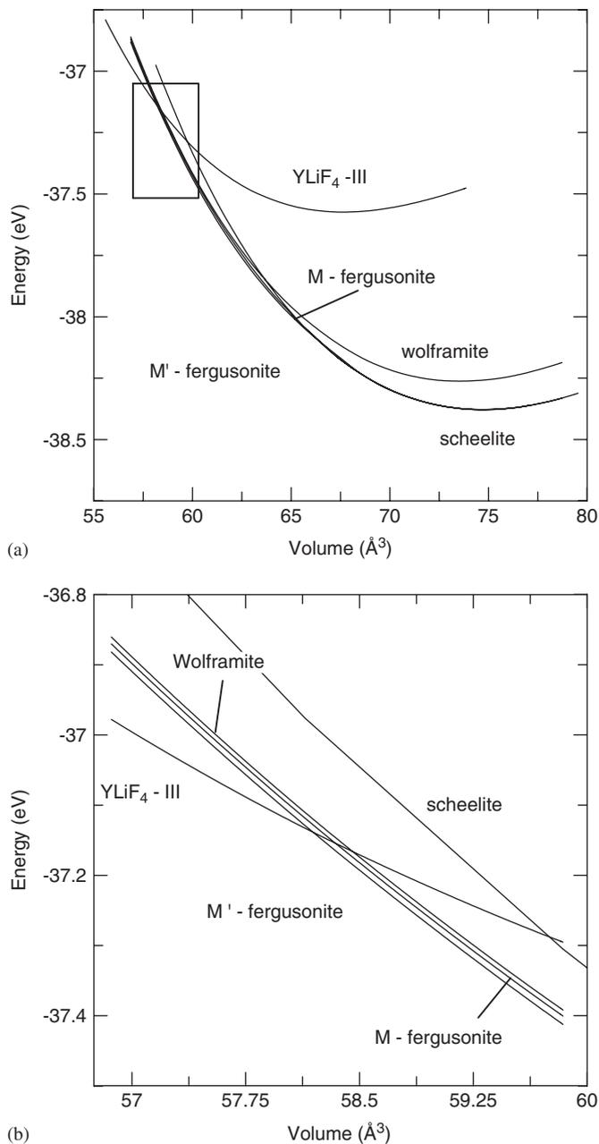
Fig. 1. (a) Energy–volume curves for some of the structures considered in this work (see text). All extensive magnitudes are written per formula unit; (b) Extended region of the second high-pressure phase transition marked in (a). The structure labelled as YLiF<sub>4</sub>-III is the high-pressure one found by Sen et al. [6].
