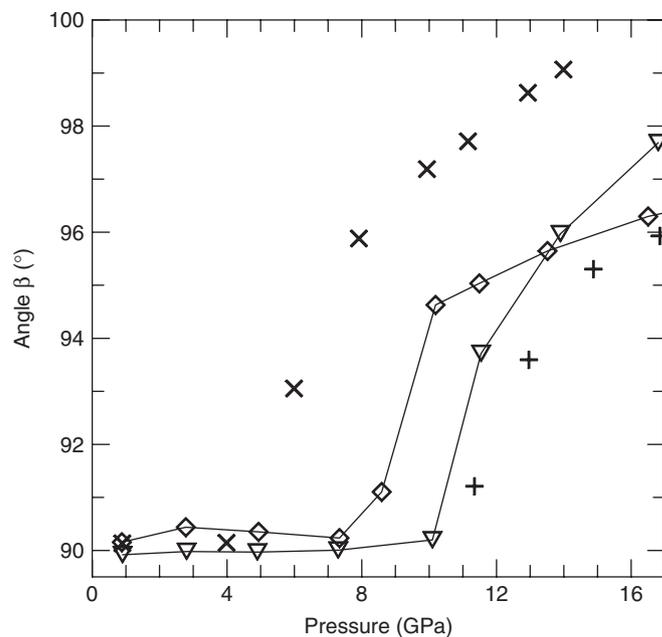
Fig. 3. Pressure dependence of the monoclinic beta angle for the M-fergusonite (triangles) and M'-fergusonite (diamonds). Experimental results after Ref. [5] (plus signs) and theoretical results after Ref. [6] (crosses) are also shown for comparison. Note that in Ref. [5] the scheelite structure, which corresponds to a beta angle of 90°, was observed till 10.6 GPa.
