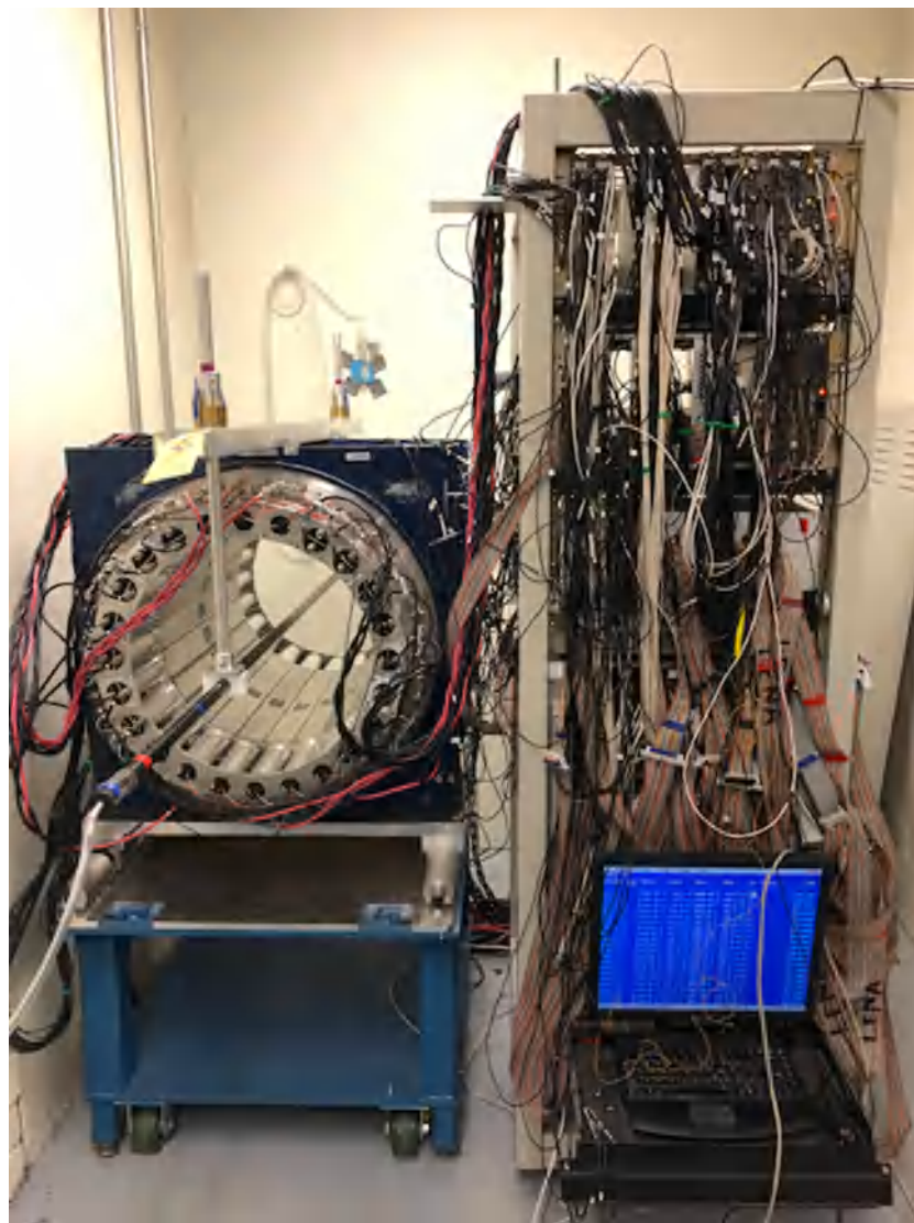
Fig. 4. The APEX array equipped with the carbon fiber tube and tubing leading to the nitrogen tank (on the left). This tubing is hooked up to a bubbler on the back wall. On the right is the DAQ and the computer that controls the PMT voltages.
