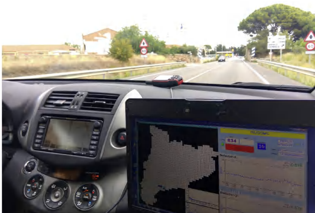
Fig. 2. Interior of the car cabin. A portable computer displays in real time the radiological data and the GPS coordinates of the last measured spectra.
