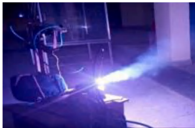
Fig. 2. A typical plasma arc photographed at the power 25 kW.
