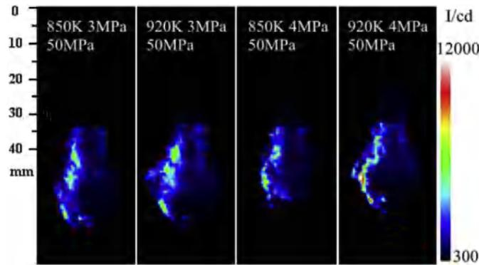
Fig. 9. Two dimensions images of LII signals at different ambient temperature and pressure.
