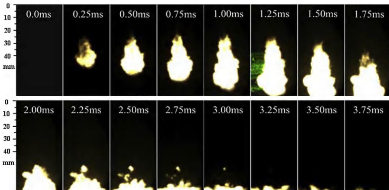
Fig. 2. Ignition process of diesel spray at diesel injection pressure 100 MPa, ambient pressure 4 MPa and ambient temperature 920 K.
