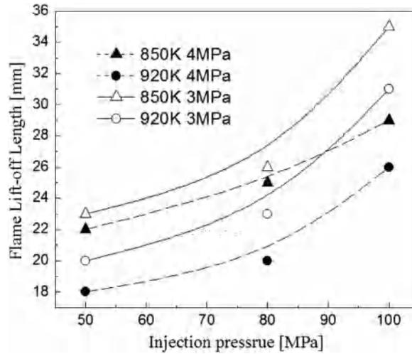
Fig. 7. Effects of different injection pressure on the flame lift-off length.
