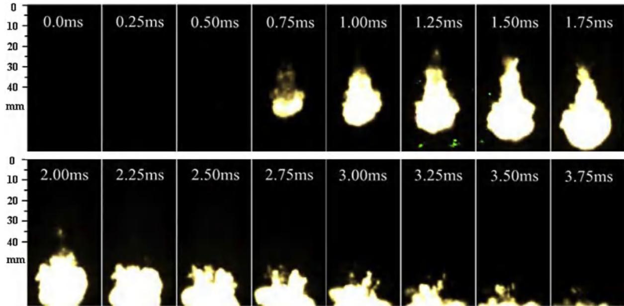
Fig. 3. Ignition process of diesel spray at diesel injection pressure 100 MPa, ambient pressure 4 MPa and ambient temperature 850 K.
