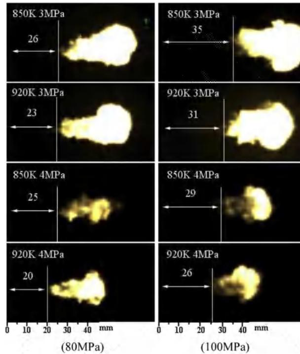
Fig. 5. Effects of different initial conditions on flame lift-off length.
