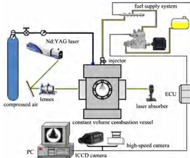
Fig. 1. Experiment measuring system of laser-induced incandescence.
