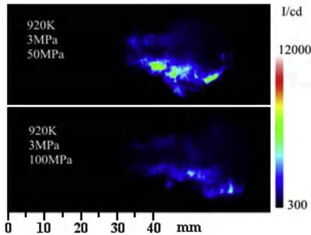
Fig. 11. Two dimensions images of LII signals at different ambient pressure and injection pressure.
