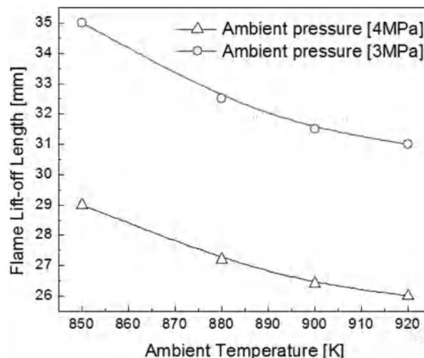
Fig. 6. The change of flame lift-off with ambient pressure and temperature.
