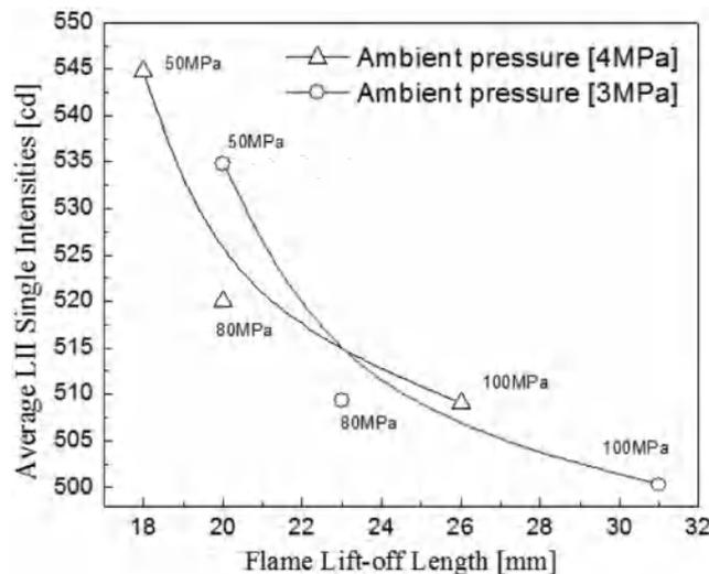
Fig. 8. LII signal intensity corresponding with different flame lift-off lengths.
