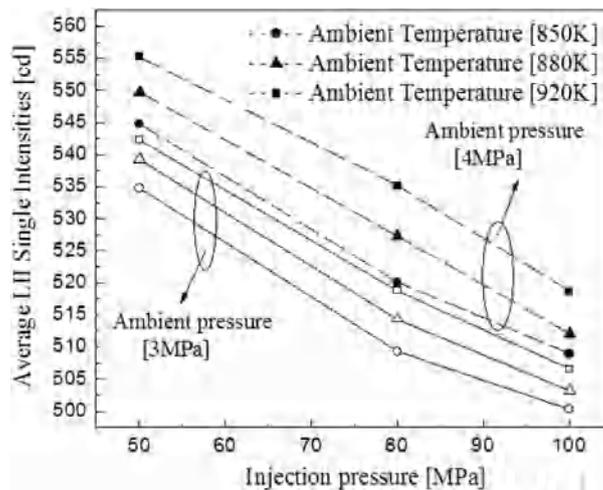
Fig. 10. Effects of different initial conditions on LII signal intensity.
