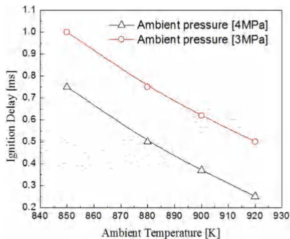
Fig. 4. Effects of different ambient pressure and temperature on ignition delay.
