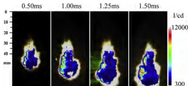
Fig. 12. Distribution of soot concentration in diesel combustion process. The 0.50 ms, 1.00 ms, 1.25 ms and 1.50 ms respectively represent the timing after start of injection of each figure.
