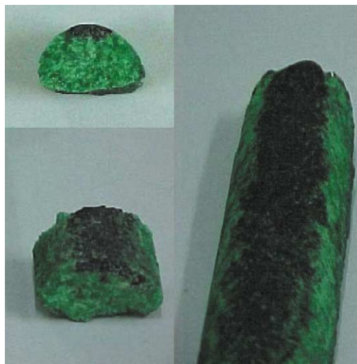
Fig. 1. Polycrystalline Cr:LiSAF ( Procedure A ) showing the dark-green phase at the bottom of the ingot resulting from \text{CrF}_3 oxidation.
