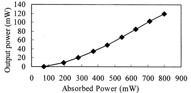
Fig. 2. Variation of output power with absorbed pump power for CW Cr:LiSGAF laser with the 1% output coupler.
