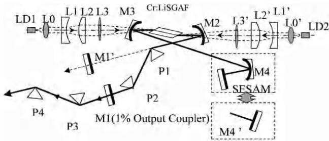
Fig. 1. Schematic of the diode-pumped self-mode-locked Cr:LiSGAF laser.
