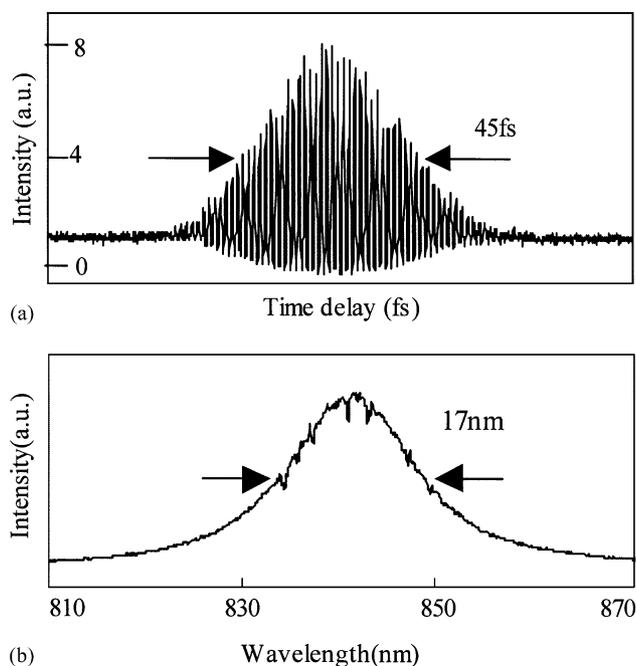
Fig. 4. (a) Interferometric autocorrelation and (b) associated spectrum of the pulse train from the Cr:LiSGAF laser.
