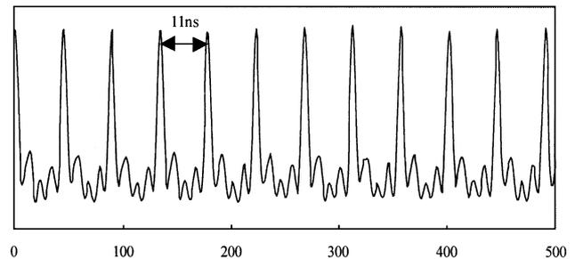
Fig. 3. Pulse train of the self-mode-locked Cr:LiSGAF laser.
