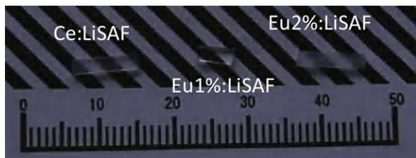
Fig. 1. View of Ce 1% (left), Eu 1% (center), and Eu 2% (right) – doped LiSAF single crystalline samples.
