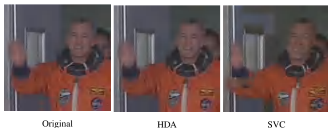
Figure 12: A part of the original frame 6 of the 4CIF Crew sequence and the versions reconstructed using the HDA and SVC schemes. (16,20) channel at 17 dB CSI-SNR.
