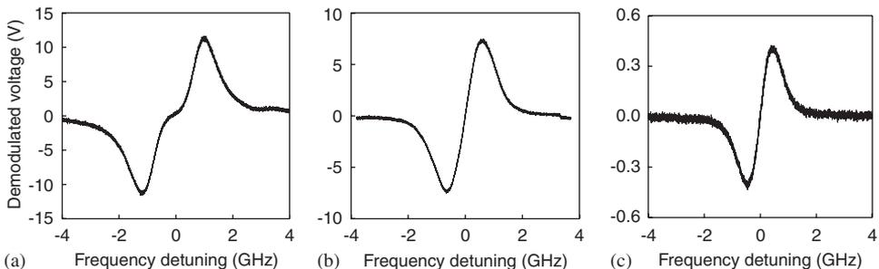
Fig. 3. FM lineshape signals corresponding to the lines shown in Fig. 3. The measurement bandwidth is 10 kHz.
