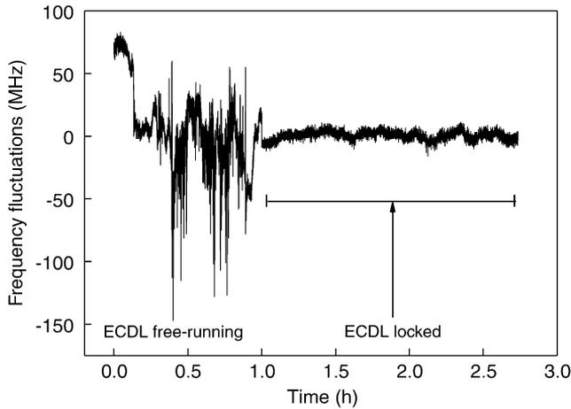
Fig. 5. Long-term frequency fluctuations as a function of the observation time when the seed laser is unlocked ( $t < 1$  h) and locked ( $t > 1$  h) to the water line at 939.710 nm.
