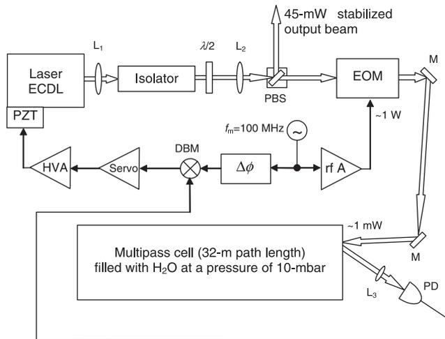
Fig. 1. Seed laser system at 935 nm. L: lens; PBS: polarizing beam splitter; EOM: electro-optic modulator; M: mirror; PD: fast photodiode; PZT: piezoelectric transducer; DBM: doubled balanced mixer; HVA: high-voltage amplifier; rf A: radio-frequency power amplifier.
