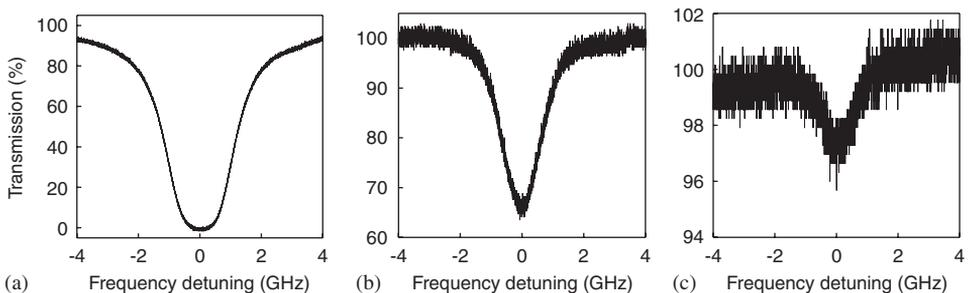
Fig. 2. Transmission spectra corresponding to three different water vapour lines at 935.684 (a), 935.299 (b), and 939.710 nm (c).
