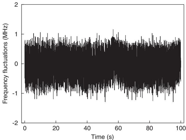
Fig. 4. Short-term frequency fluctuations as a function of the observation time when the seed laser is locked to the water line at 935.299 nm. The sampling period was 10 ms.
