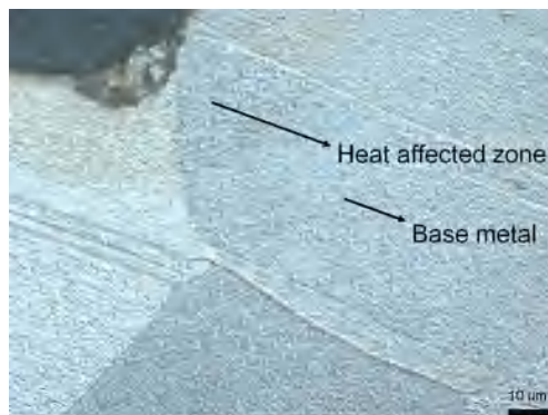
Fig. 25.10 Differential Interference Contrast micrograph showing the microstructural changes of a laser machined Incoloy 800 HT superalloy etched with marbles [34].
