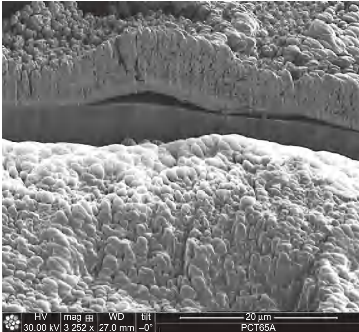
Fig. 25.17 Cross-section SEM micrograph of the laser-machined 316LVM by Nd:YAG laser. Grains of several micrometers ( 2.23 \mu\text{m} \pm 0.34 \mu\text{m} ) are observed by ion-induced secondary electron imaging [34].
