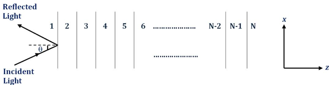
Fig. 2. Schematic for N-layer transfer matrix method to calculate the reflected light intensity (R).
