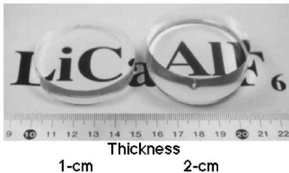
Fig. 7. Wafers cut perpendicular to the growth axis of the undoped LiCaAlF 6 single crystal.
