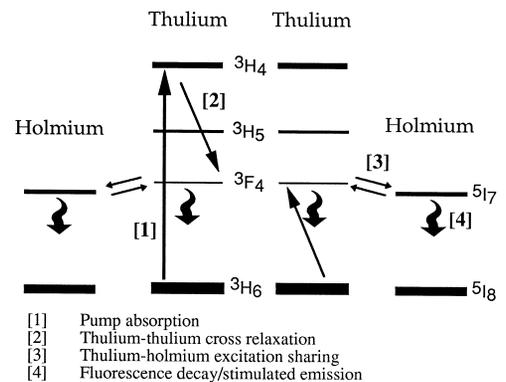
Fig. 2. Excitation mechanisms in diode-pumped two micron lasers.
