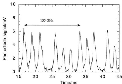
Fig. 11. Fabry-Perot trace of Tm,Ho:YAP laser output.
