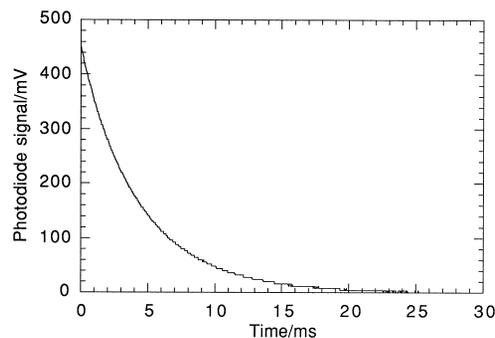
Fig. 8. Infrared fluorescence decay of Tm:YAP.
