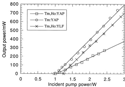
Fig. 4. Best output power performance of the three lasers.
