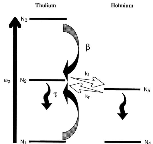
Fig. 16. Principal parameters used in relaxation oscillation analysis.
