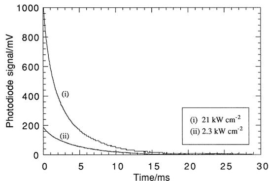
Fig. 7. Intensity-dependent fluorescence decay profiles of Tm,Ho:YAP.
