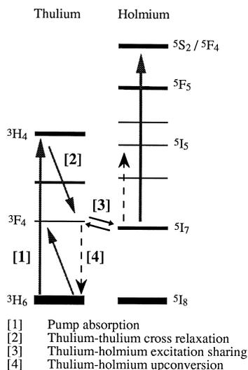
Fig. 6. Principal upconversion mechanisms in double-doped materials.
