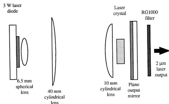
Fig. 3. Schematic of laser experimental set-up.
