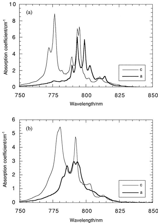
Fig. 1. Pump band absorption spectrum of (a) 4.2% thulium in YAP, and (b) 6% thulium in YLF.
