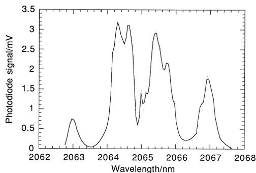
Fig. 12. Spectrum of Tm,Ho:YLF laser output.
