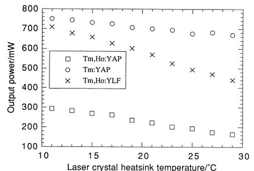
Fig. 5. Comparison of temperature dependence of output power.
