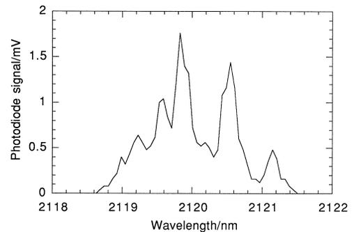
Fig. 10. Spectrum of Tm,Ho:YAP laser output.
