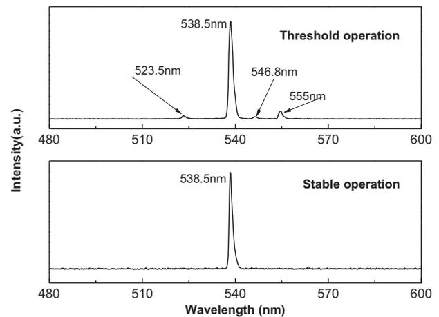
Fig. 6. Visible laser spectra generated from frequency mixing in KTP crystal.
