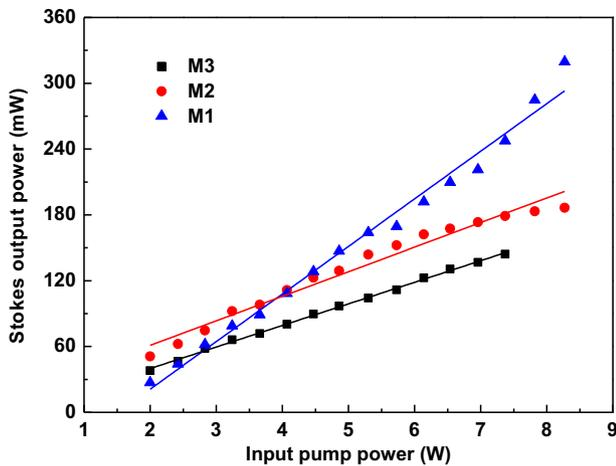
Fig. 3. Stokes wave output power versus input pumped power with different output couplers.
