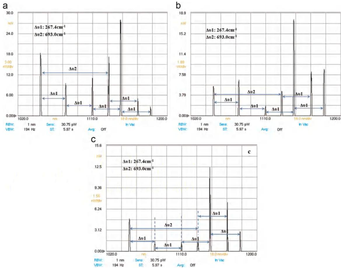
Fig. 2. Output spectra of the KTP Raman laser with different output couplers M1 (a), M2 (b) and M3 (c).
