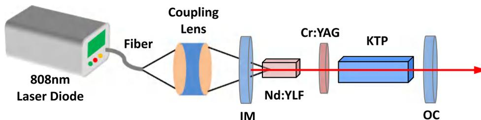
**Fig. 1.** Experimental setup of the multi-wavelength KTP Raman laser.
