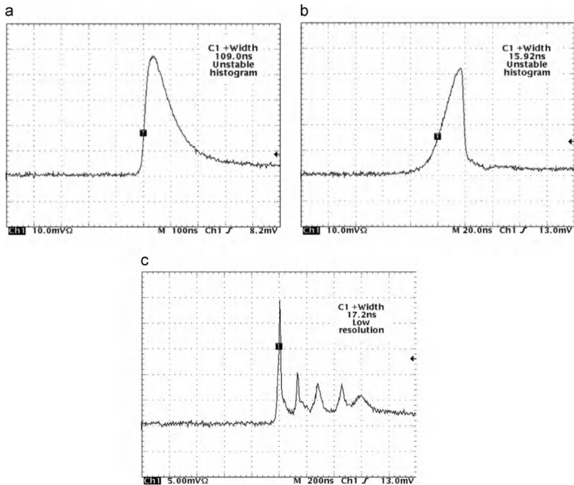
Fig. 4. Temporal pulse shapes of the free-running fundamental wave (a), depleted fundamental wave (b) and Stokes waves (c).
