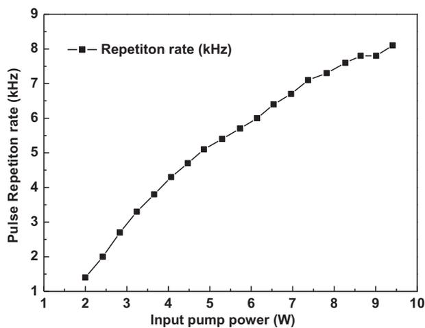
Fig. 5. Repetition rate versus input pump power.
