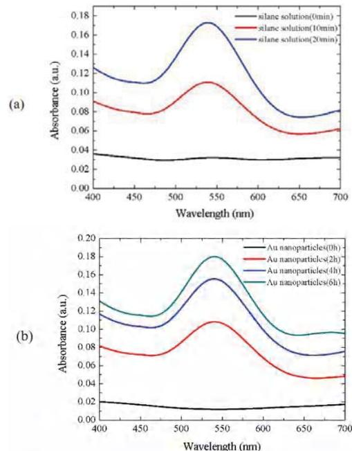
Figure 2. (a) The relationship between the interact time of the SU-8 polymer film with the silane solution and the absorbance of the polymer film coated with gold nanoparticles; (b) The relationship between the interact time of the SU-8 polymer film with the nanoparticles solution and the absorbance of the SU-8 polymer film coated with gold nanoparticles.
