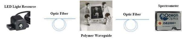
Figure 5. Schematic of measurements setup.
