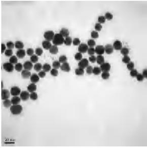
Figure 1. TEM image of gold nanoparticles.
