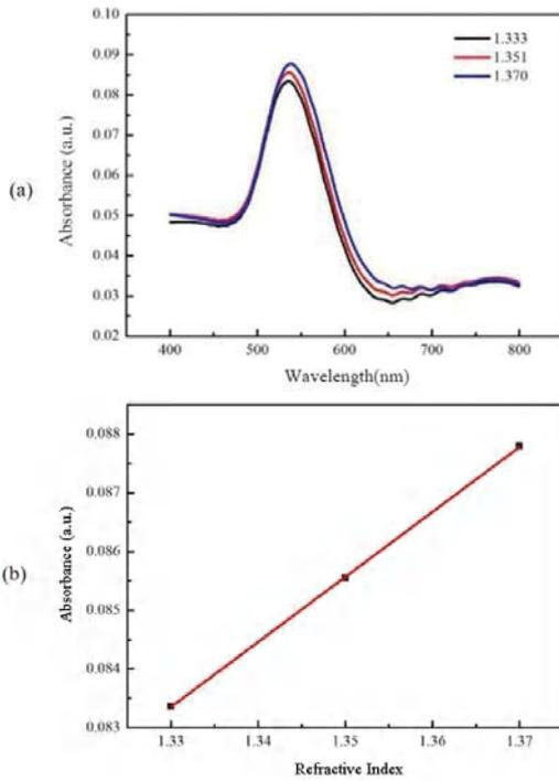
Figure 3. (a) The normalized absorbance spectrum of the polymer film exposed to different concentrations of NaCl solution with the refractive index between 1.333 and 1.370; (b) The linear relationship between the refractive index of NaCl solution and the absorbance of the polymer film coated with gold nanoparticles.
