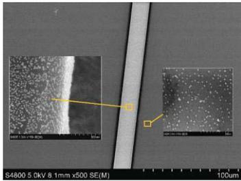
Figure 4. The SEM images of polymer waveguide coated with gold nanoparticles.
