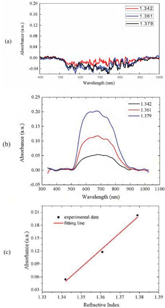
Figure 6. The normalized absorbance spectrum of the polymer waveguide without gold nanoparticles for detecting different concentrations of NaCl solution; (b) The normalized absorbance spectrum of the polymer waveguide coated with gold nanoparticles for detecting different concentrations of NaCl solution; (c) The linear relationship between the refractive index of NaCl solution and the absorbance of the polymer waveguide coated with gold nanoparticles.
