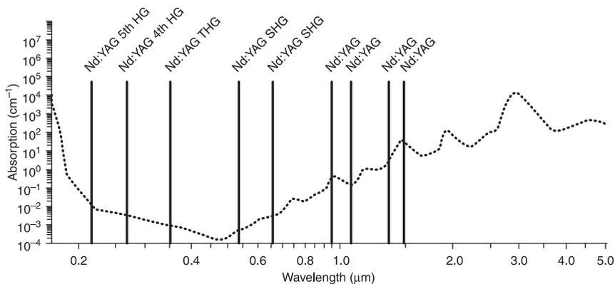
5.11 Nd:YAG laser emission and its harmonics on the basis of the absorption of radiation in water.
