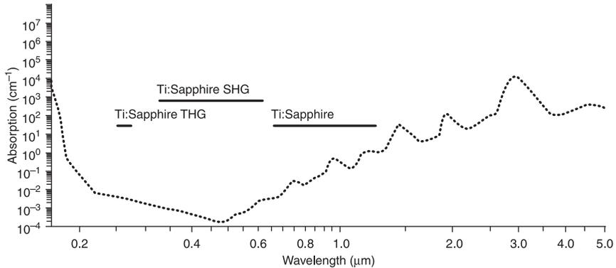
5.10 Ti:Sapphire emission on the basis of the absorption of radiation in water.
