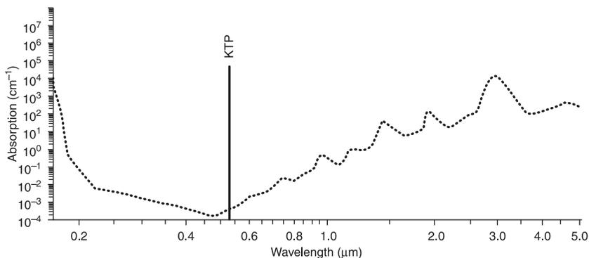
5.12 Wavelength generated by Nd:YAG/KTP laser on the basis of the absorption of radiation in water.
