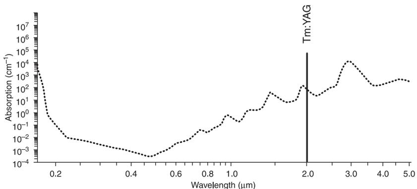
5.14 Tm:YAG laser emission on the basis of the absorption of radiation in water.
