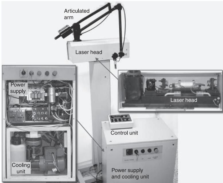
5.2 Schematic of solid-state laser systems (dental laser driller).
