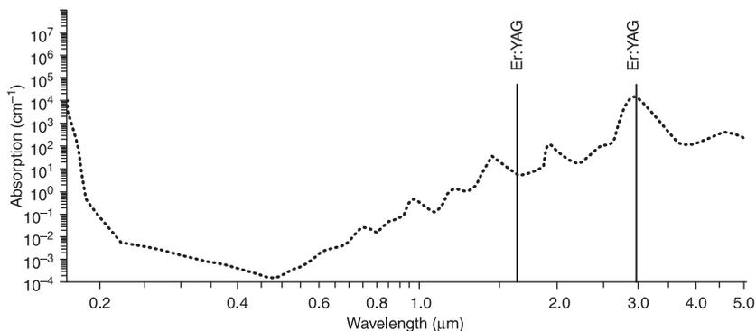
5.13 Er:YAG laser emission on the basis of the absorption of radiation in water.
