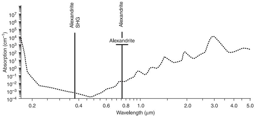
5.9 Alexandrite laser emission on the basis of the absorption of radiation in water.
