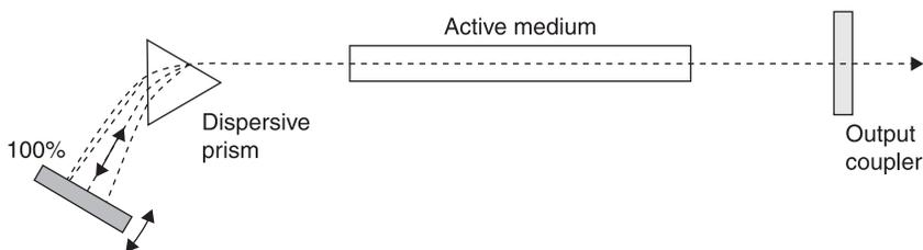
5.7 The scheme of laser resonator tuned using a dispersive prism.
