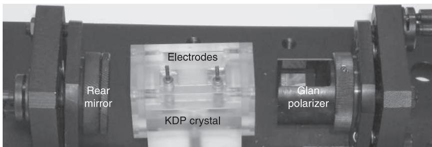
5.6 Photograph of the electro-optical Q-switch – Pockels cell – operated at a quarter-wave retardation voltage.
