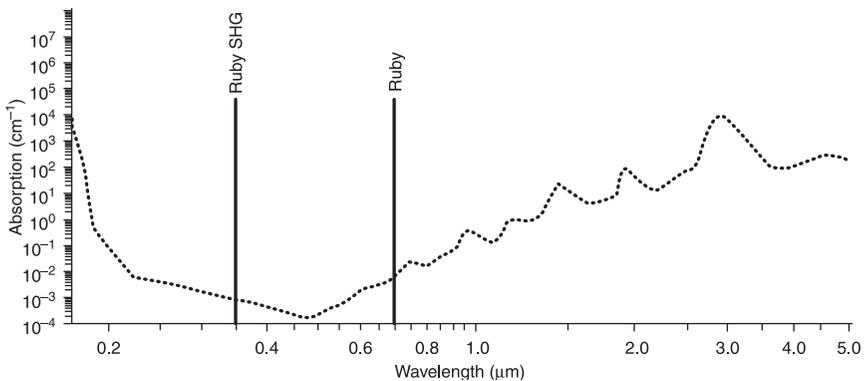
5.8 Ruby laser emission on the basis of the absorption of radiation in water.
