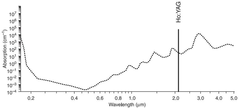
5.15 Ho:YAG laser emission on the basis of the absorption of radiation in water.
